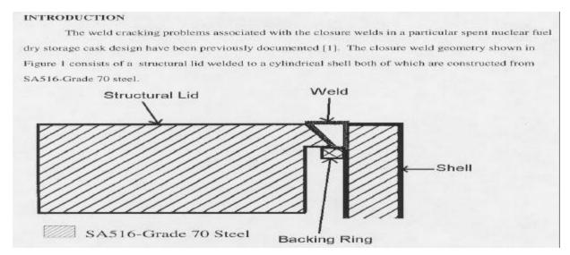
pre-service examination. Since a particular material can exist in many different grades and classes, it is crucial that the exact class and grade of material to be used to fabricate a DCSS be properly tested and evaluated for regulatory requirements.
