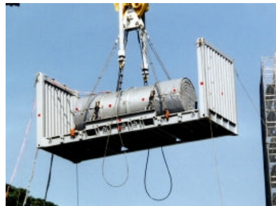
Fig.10 Insulated 48Y-cylinder Equipped with the Japanese Heat-Protective Covers
