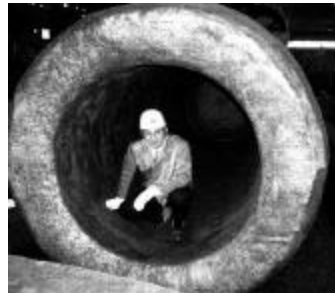
Fig. 2 Monolithic forging for MSF cask
