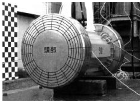
Fig.7 1/2 Scale model for drop test
