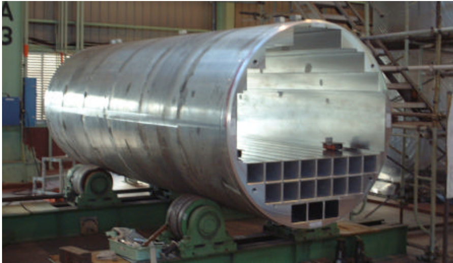
Figure7, Assembling Square Tubes and Neutron Absorbing Materials in the Aluminum Block
