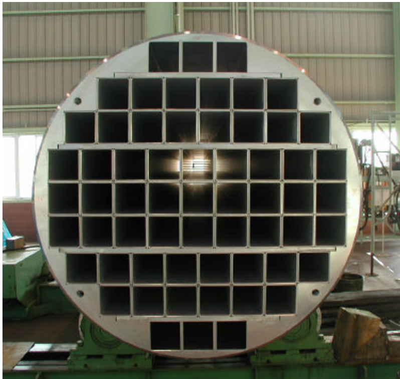
Figure8, Completed Fuel Basket
