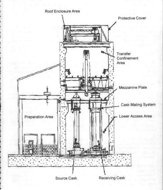
Confinement Area. When the spent fuel transfer tube is aligned with the receiving cask, the device opens and any accumulated crud falls into the receiving cask, e.g., the MPC. There will be two monitoring systems in the facility to ensure proper grappling of the fuel: (1) a video monitor and (2) a series of switches, to assure that the operator knows the position of the fuel at all times. The fuel handling machine can be operated manually from the facility catwalks for off-normal recovery.
