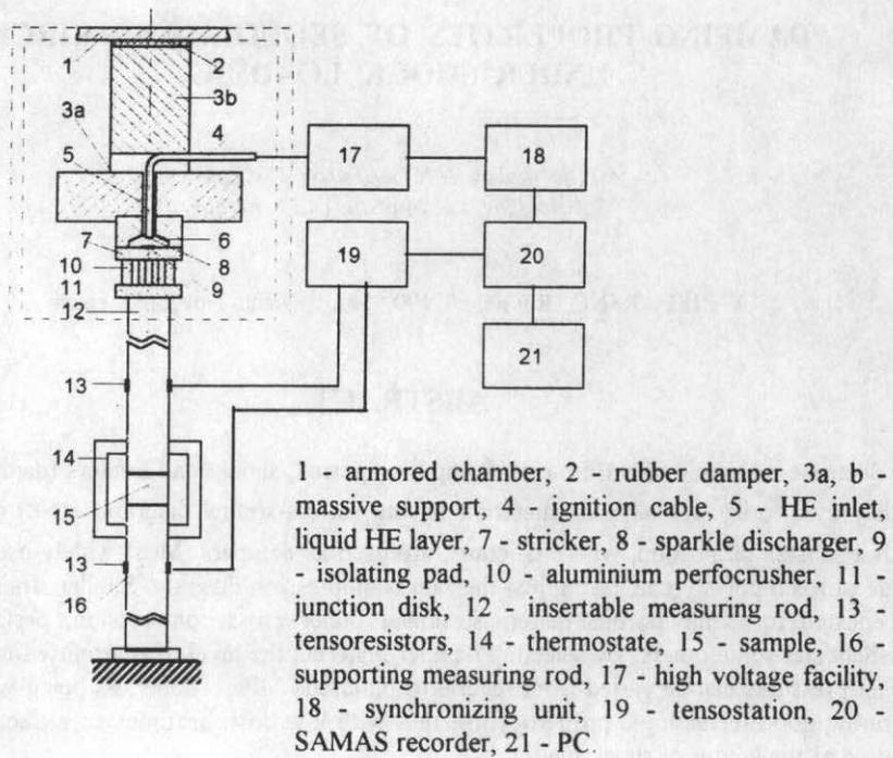
Fig. 1. Schematic layout of measuring/computation complex.
