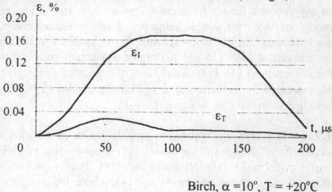
Fig. 2. Recording of strains in loading ( $\epsilon_i$ ) and passing ( $\epsilon_T$ ) waves of stress.
