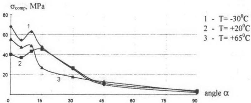
Fig. 5. Sequoia strength  $\sigma_{comp}$  vs angle  $\alpha$  and temperature.
