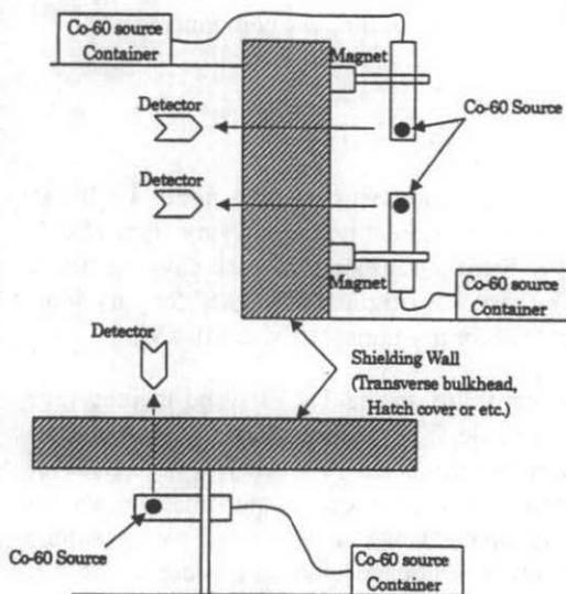
Fig. 7 General arrangement of the Shielding Test-1
