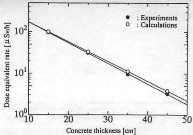
Fig. 4 Comparison of the experiments and calculations (neutron dose equivalent rates)
