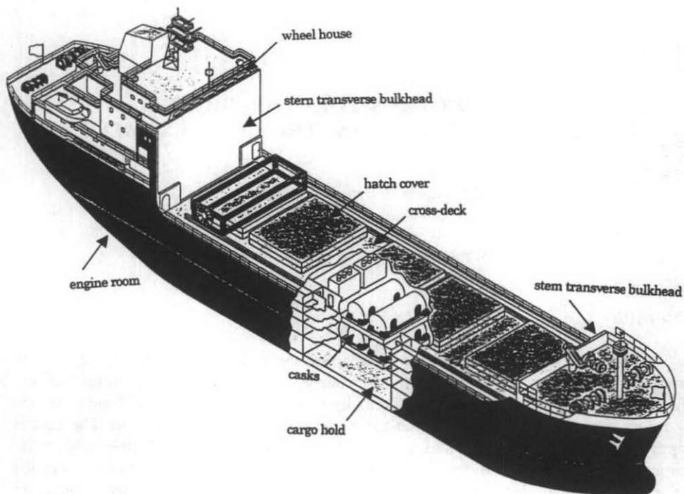
Fig. 6 Overview of the ship's shielding structure
