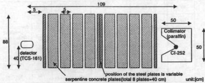
Fig. 3 Experiment arrangement for secondary gamma-ray (Ci-252)
