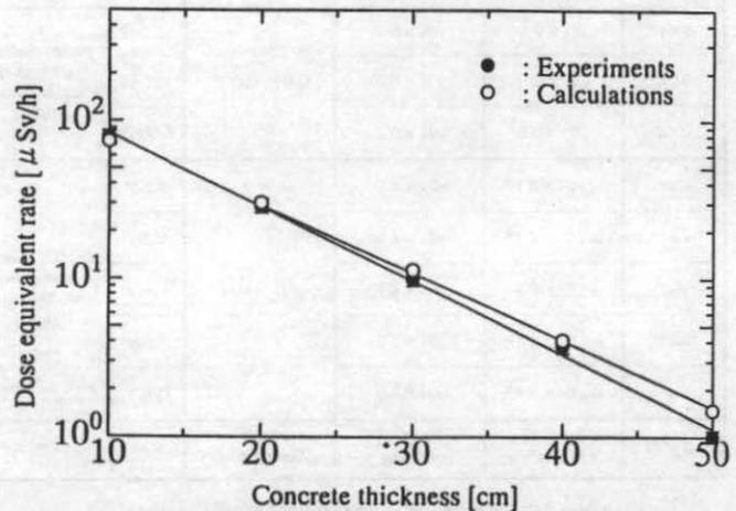
Fig. 5 Comparison of the experiments and calculations (gamma-ray dose equivalent rates)
