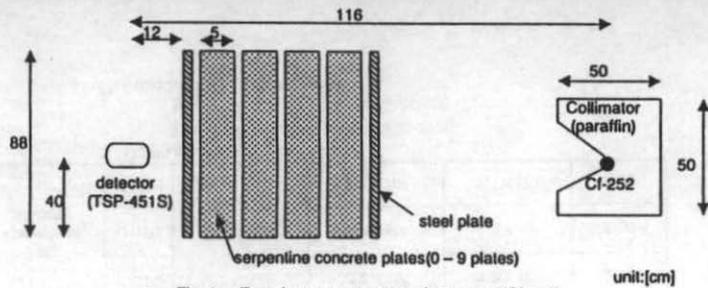
Fig. 1 Experiment arrangement for neutron (Ci-252)
