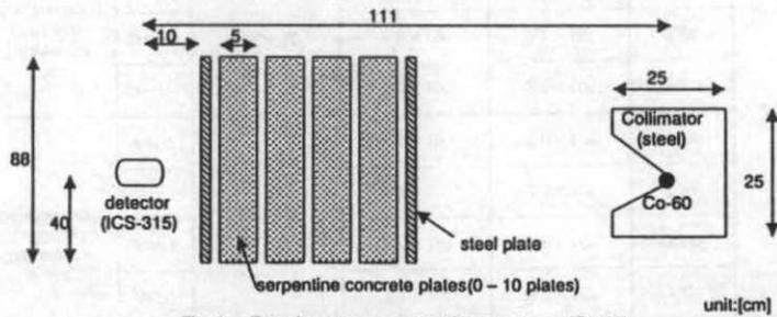
Fig. 2 Experiment arrangement for gamma-ray (Co-60)
