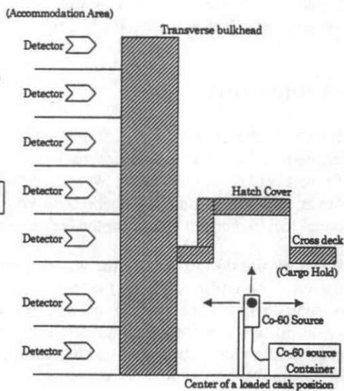
Fig. 8 General arrangement of the Shielding Test-2
