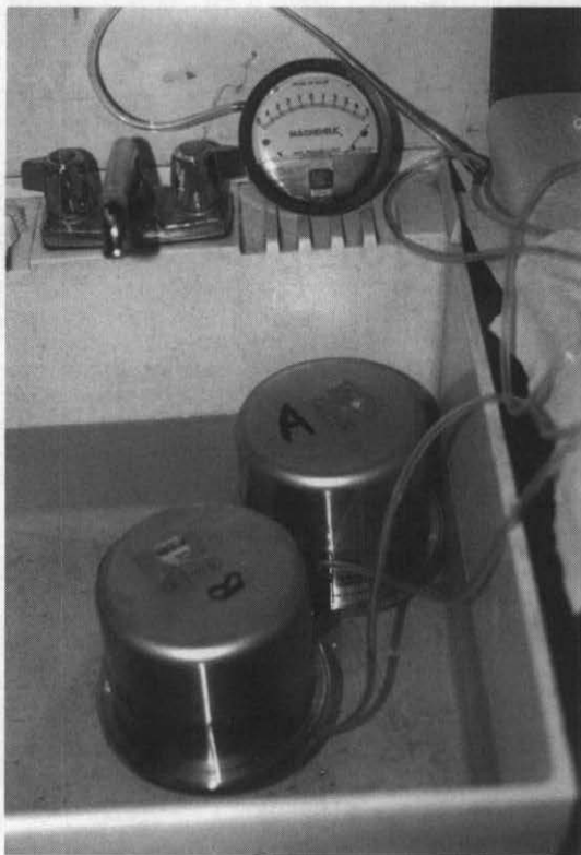
Figure -4 Pressurized Leak Test
