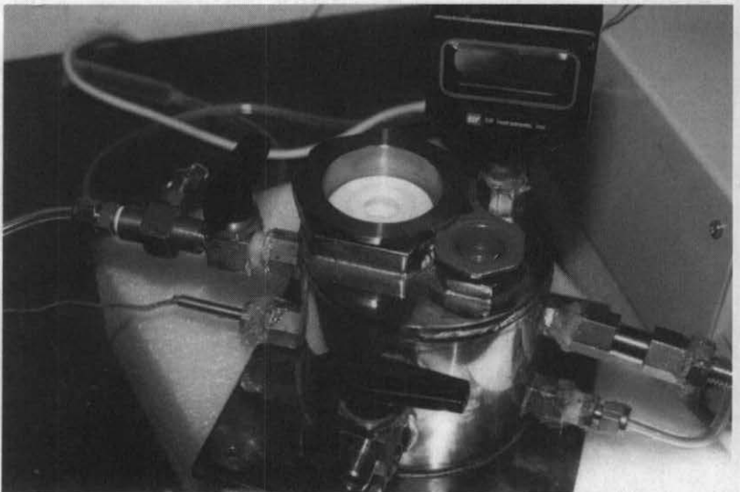
Figure -6 Test chamber for hydrogen diffusion measurements
