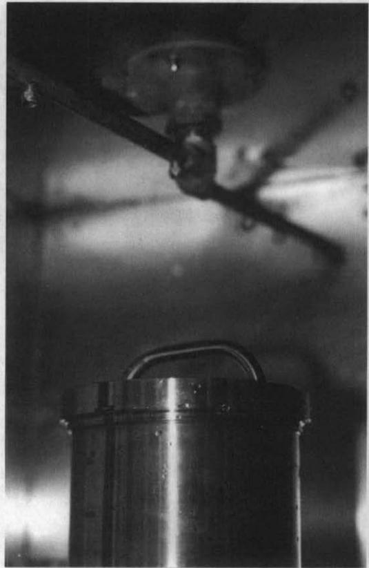
Figure -10 NMC in high pressure industrial water spray test
