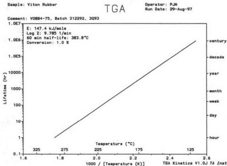
Figure 3. Predicted lifetime plot for Viton® rubber at 1% conversion in air.
