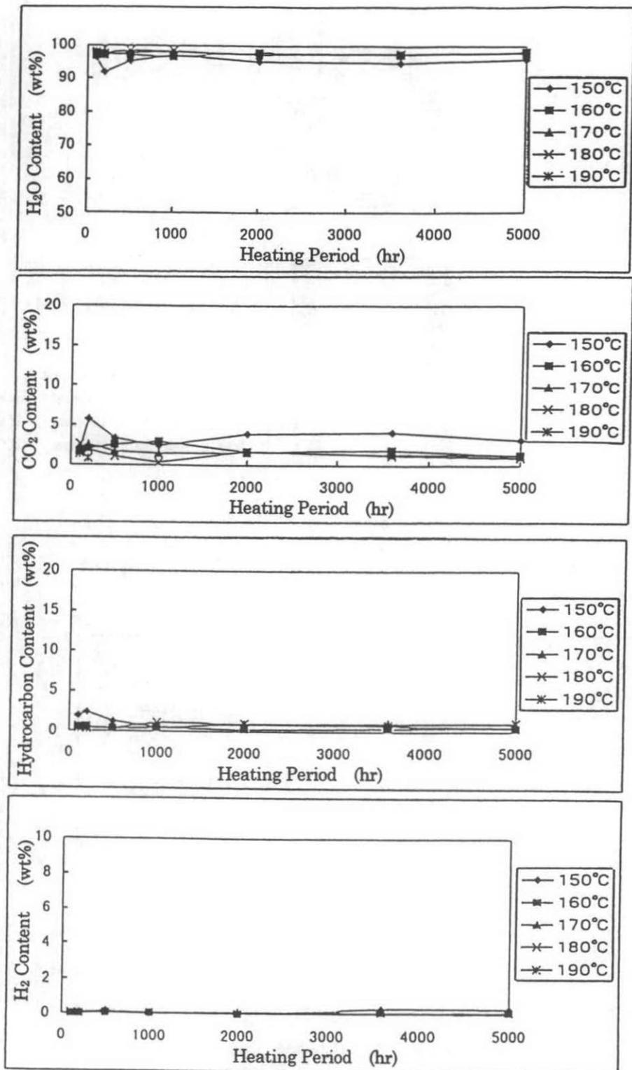
Figure 1-3 Content of Gaseous Compound released by Heating
