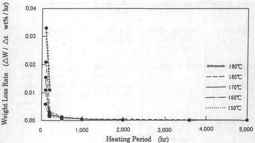
Figure 1-2 Change of Weight Loss Rate
