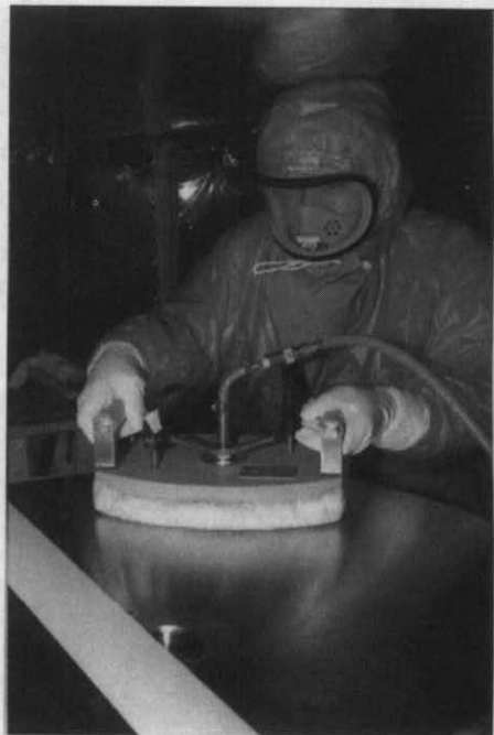
Buffer treatment of an internal thread on the packaging upper section
