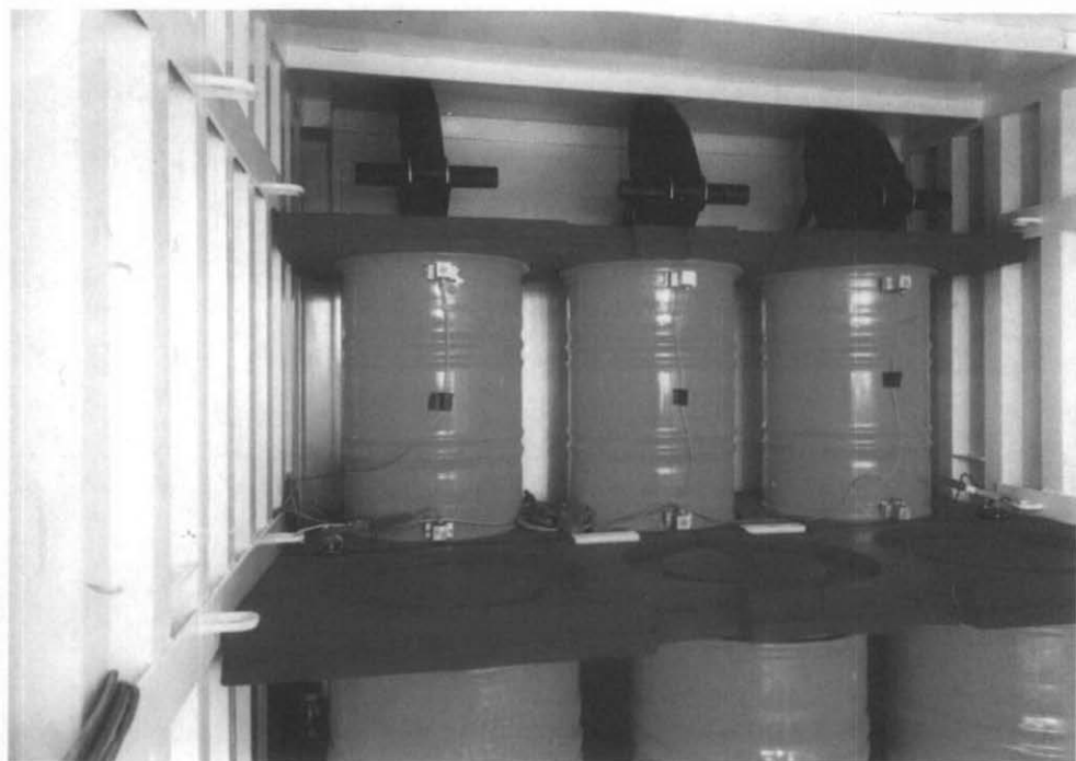
Figure 2. The BOXFORCE ® Container being Loaded with 200 liter Drums Showing the Elasto-Plastic Support Trays
