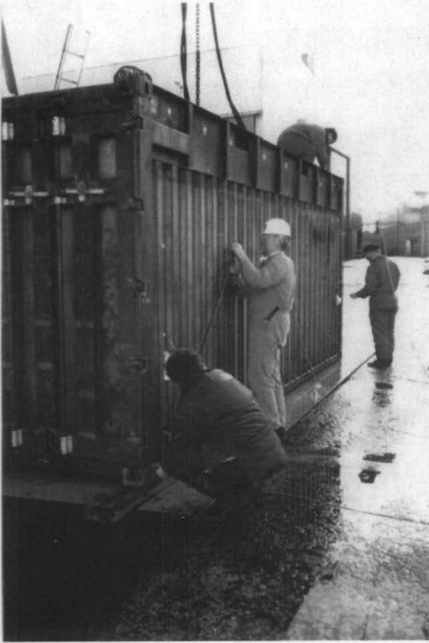
Figure 3. The BOXFORCE ® Container after the 0.3 m Drop Test
