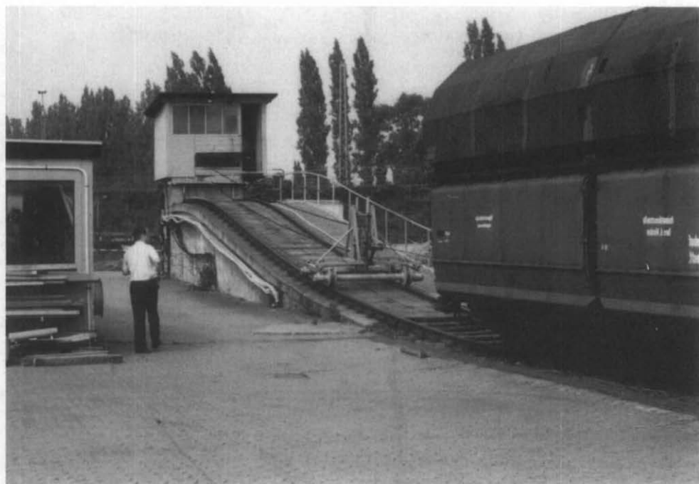
Figure 4. Testing Facilities of the German Railway in Minden/Germany Showing Ram Car and Ramp Pull-up Winch
