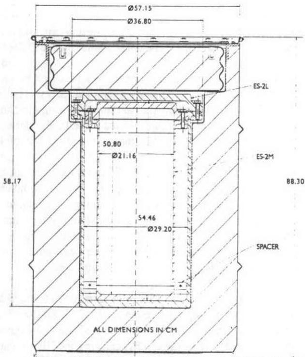
Fig. 1. A schematic view of the ES-2LM test package
