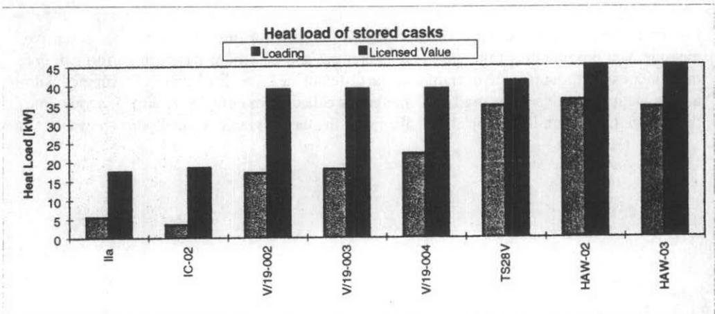
Fig. 3 - Heat load of the stored casks
