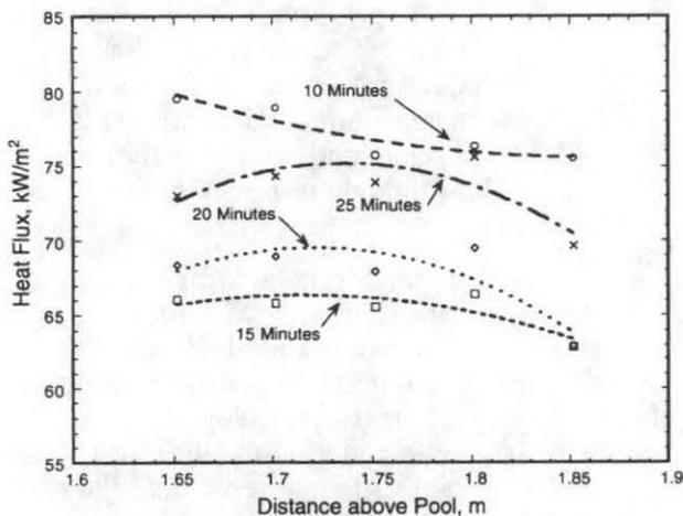
Figure 6. Heat flux vs. Distance above pool for second test with calorimeter at center of pool.
