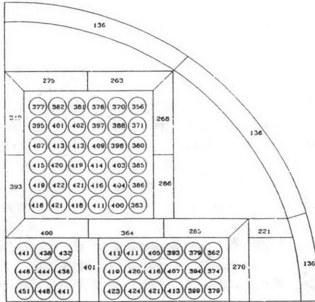
Fig. 7. Temperature Distributions of Fuel Assemblies in Air Cavity
