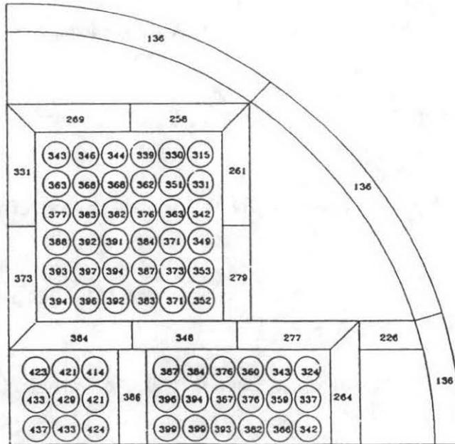
Fig. 8. Temperature Distributions of Fuel Assemblies in Helium Cavity
