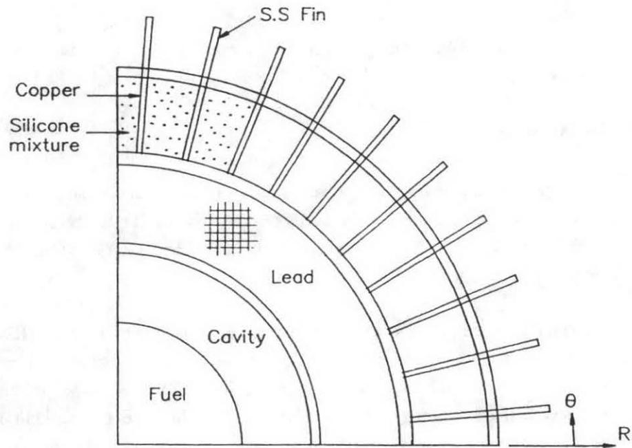
Fig. 5. Thermal Analysis Model for Slice Model
