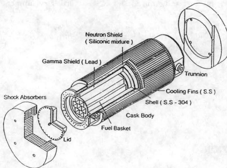
Fig. 1. Configuration of KSC-7 Shipping Cask
