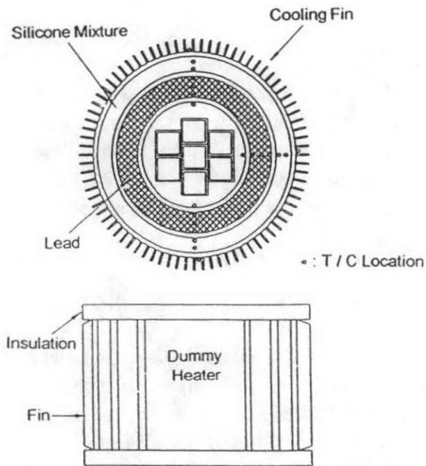
Fig. 2. Slice Model of KSC-7 Cask
