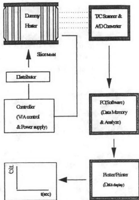
Fig. 3. Temperature Measuring System
