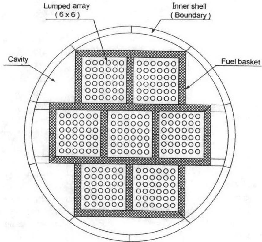
Fig. 6. Subchannel Thermal Analysis Model for Fuel Assemblies
