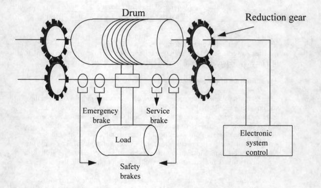
Moreover the lifting motion is controlled by two electronic systems instead of one before. The first one performed the following functions: power misfit, sensor fault, drum rotation fault, low speed and high speed overspeed, low speed and high speed redundancy, failure in kinematic chain, static veering and dynamic veering.
