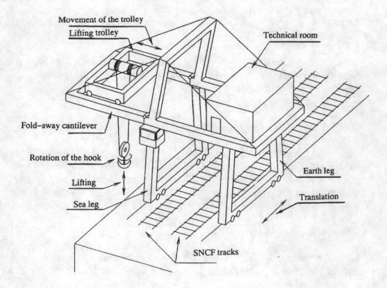
The gantry crane is composed of two legs, on the sea and land side, which have two articulated and motorized bogies, rolling on the two tracks. These legs ensure thus a translation movement to the gantry crane along the wharf and allow it to be positioned at the base of the unloaded ship decks.
