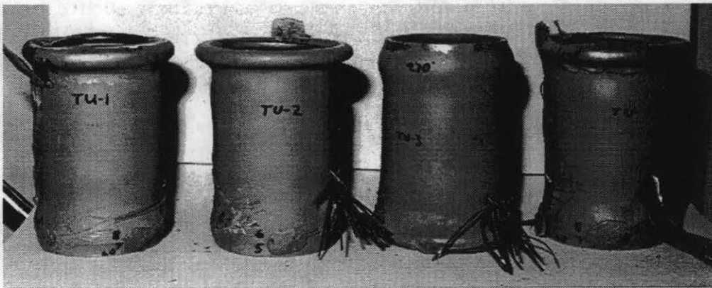
Figure 3. Deformed shape for the four test articles.
