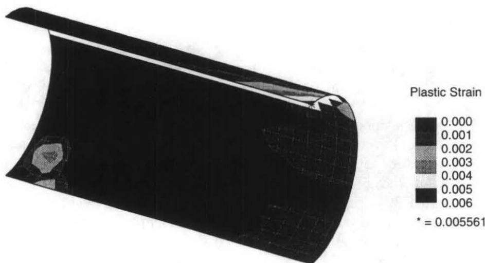
Figure 4. Strains predicted from nonlinear dynamic analysis of the ferritic steel package with 0.25 inch thick wall
