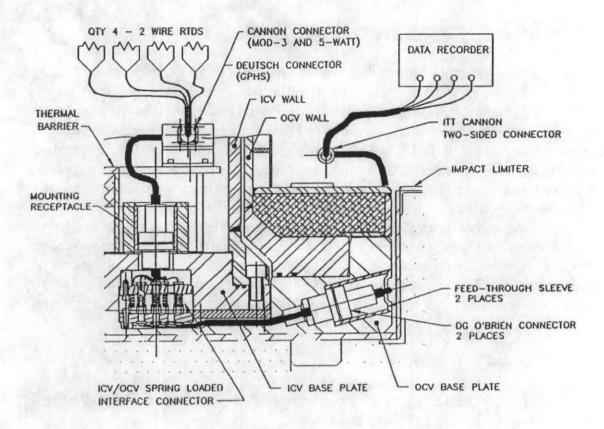
Figure 3. Electrical Feed-Through Design Feature.
