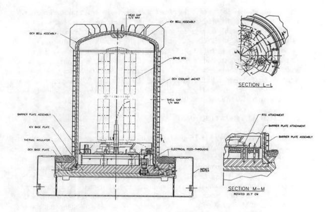
Figure 2. RTG Transportation Package With GPHS Payload.
