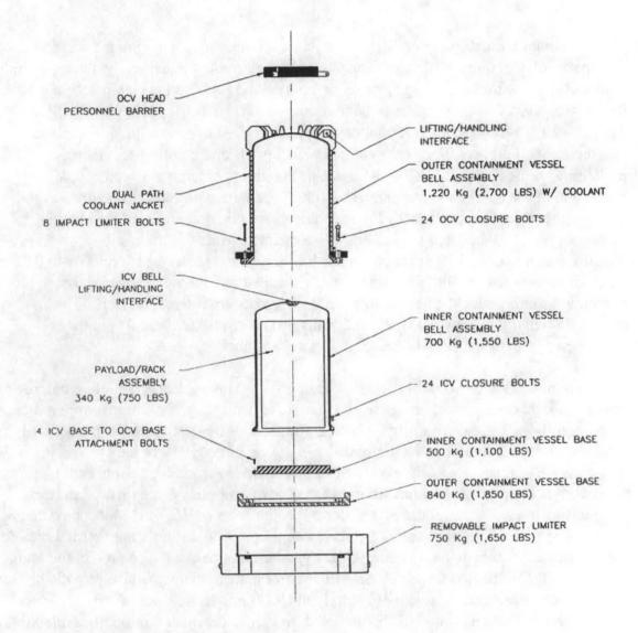
Figure 1. RTG Transportation Package.
