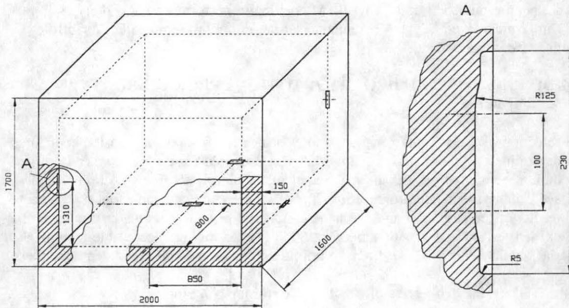
**Figure 2. Geometry of the Artificial Flaw-Like Defects**
