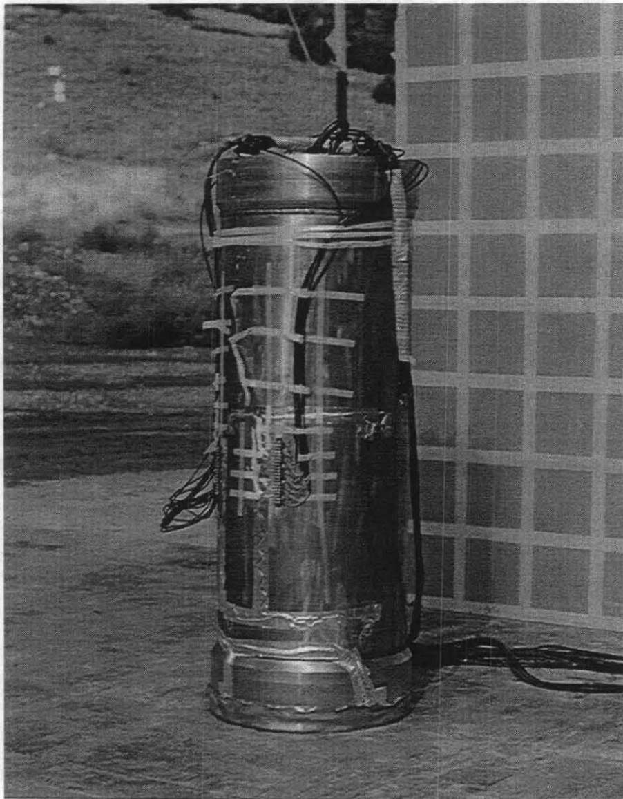
Figure 2. SETU test unit after impacting unyielding target.
