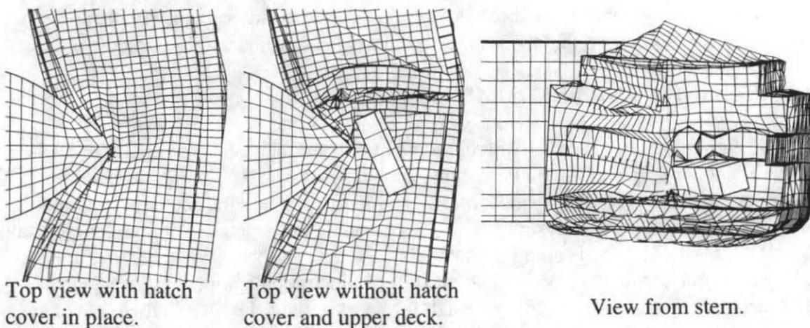
**Figure 3.** Maximum deformation for Case 4S ( $v = 30$  knots, mass = 16,750 tonnes,  $t = 0.68$  seconds).
