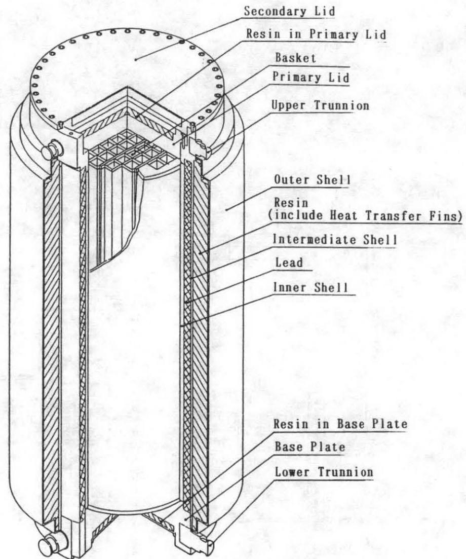
Figure 1 Hitachi Zosen's Dry Storage Cask
