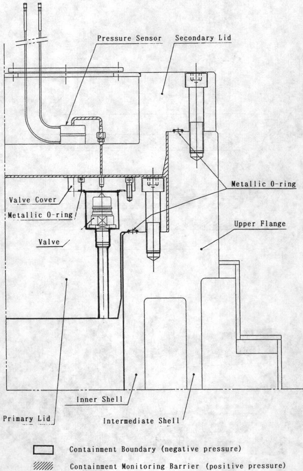
Figure 2 Detail of Containment Boundary and Monitoring System
