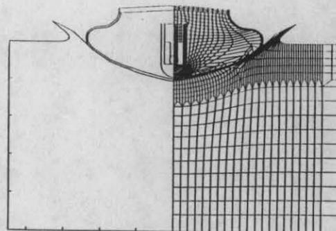
Figure 5 Finite element simulation result of test package impact on grout.
