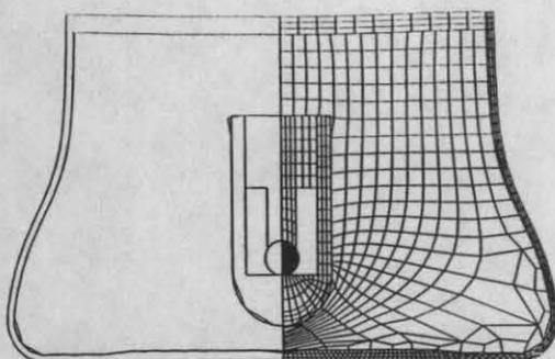
Figure 4 Finite element simulation result of test package impact on steel plate.
