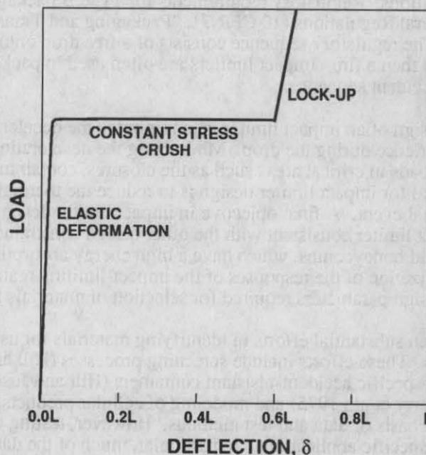
Figure 1. Idealized Crush Load-Deflection Curve
