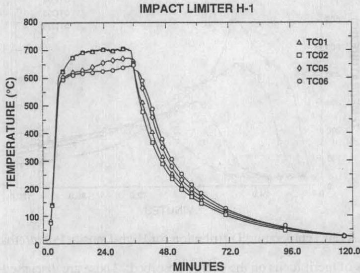
Figure 5. Axial Temperature Distribution for Aluminum Honeycomb
