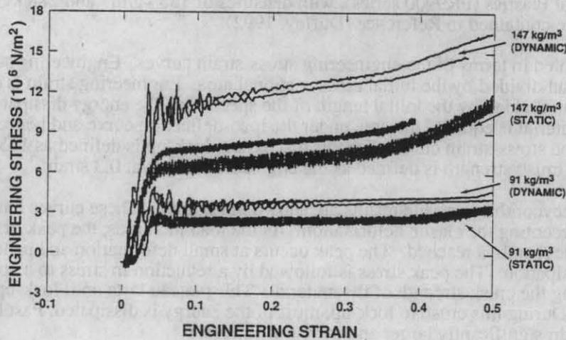
Figure 3. Polyurethane Foams Composite Results
