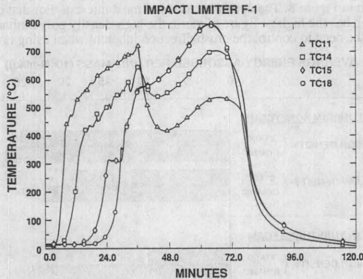
Figure 6. Axial Temperature Distribution for Low-Density Polyurethane Foam
