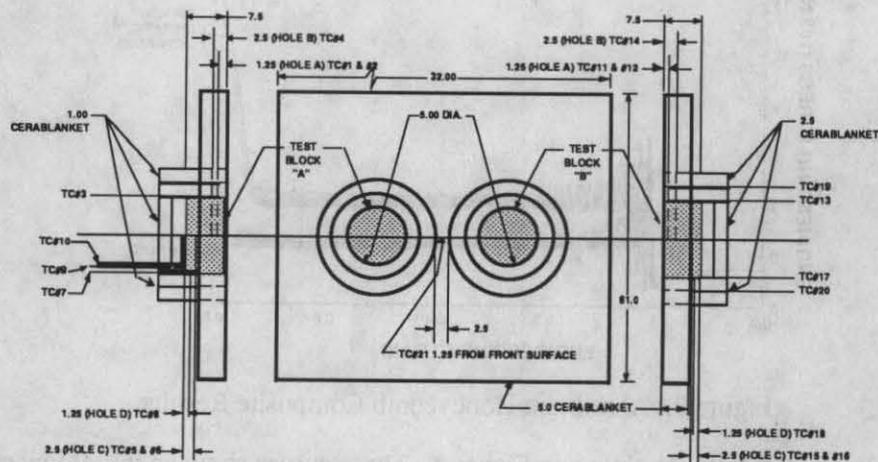
Figure 4. Thermal Test Setup
