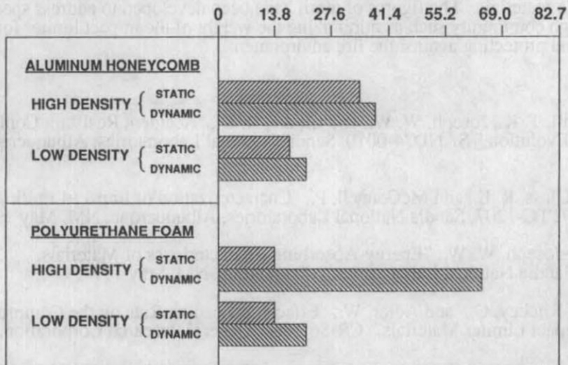
Figure 10. Energy Absorbed per Unit Volume Using Janssen Factor
