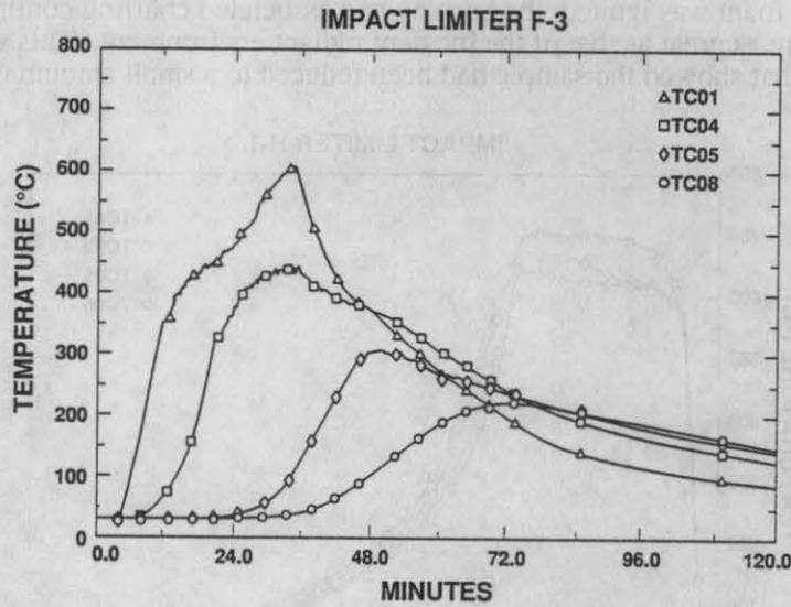
Figure 7. Axial Temperature Distribution for High-Density Polyurethane Foam
