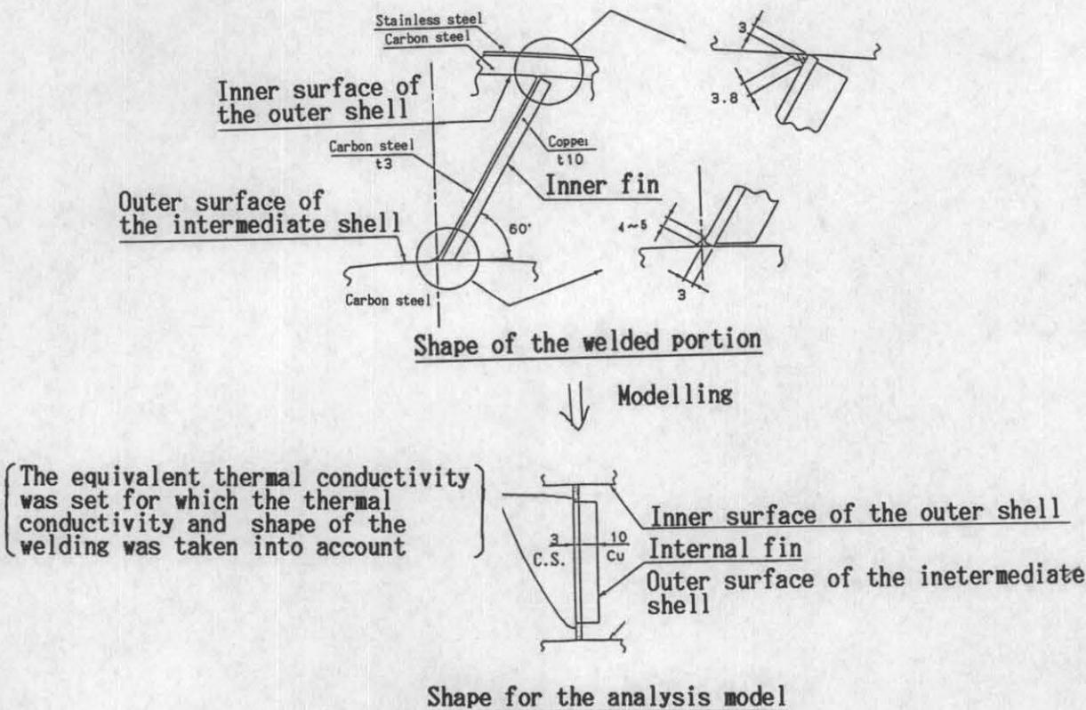
Fig. 11 Modelling of the welded portions of the internal fins
