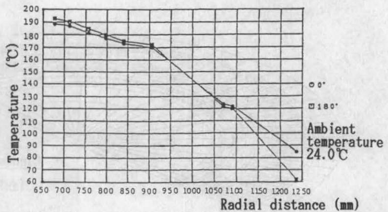
Fig. 6 Radial Temperature Distribution
