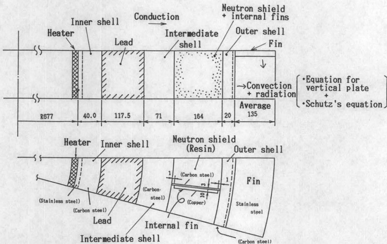
Fig. 10 Concept adopted for heat transfer in the analysis
