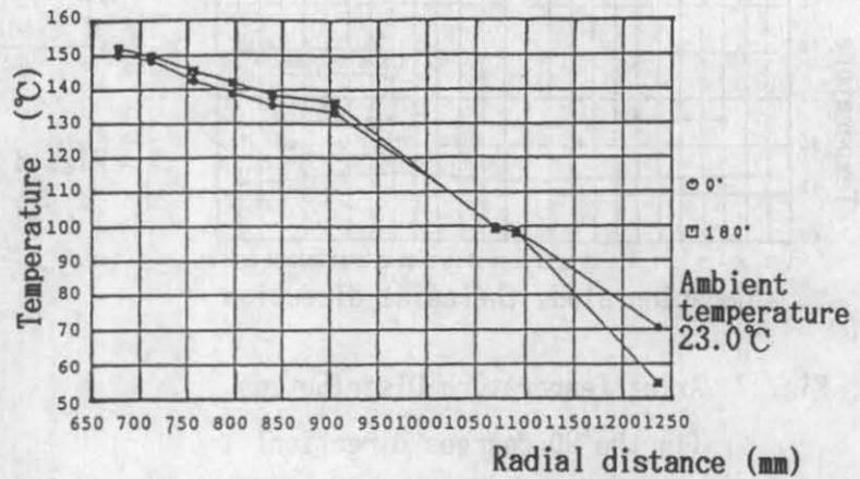
Fig. 5 Radial Temperature Distribution
