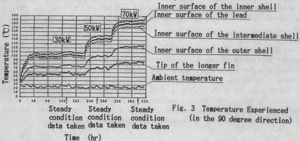
Fig. 3 Temperature Experienced (in the 90 degree direction)
