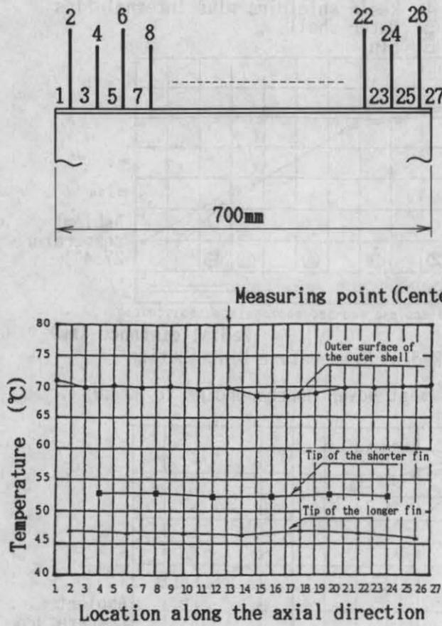
Fig. 7 Axial Temperature Distribution
