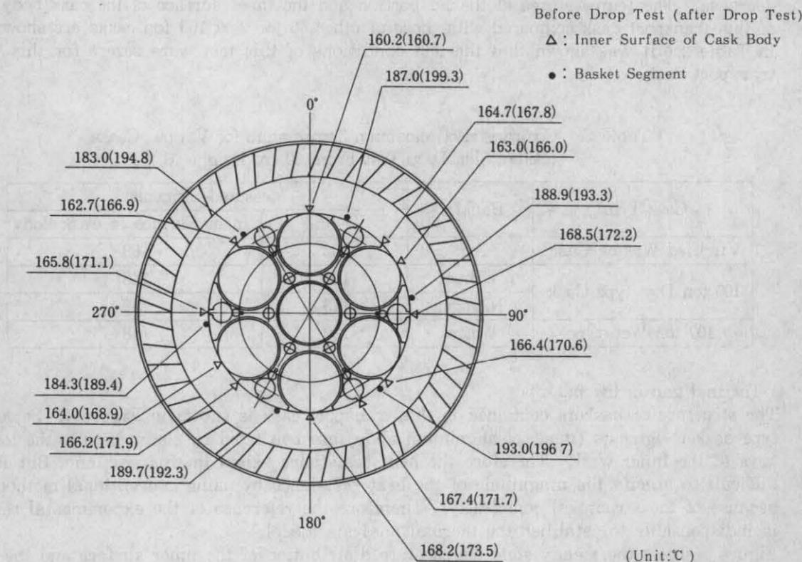
Figure 5. Thermal Gap Between Basket and Inner Surface of Cask Body
