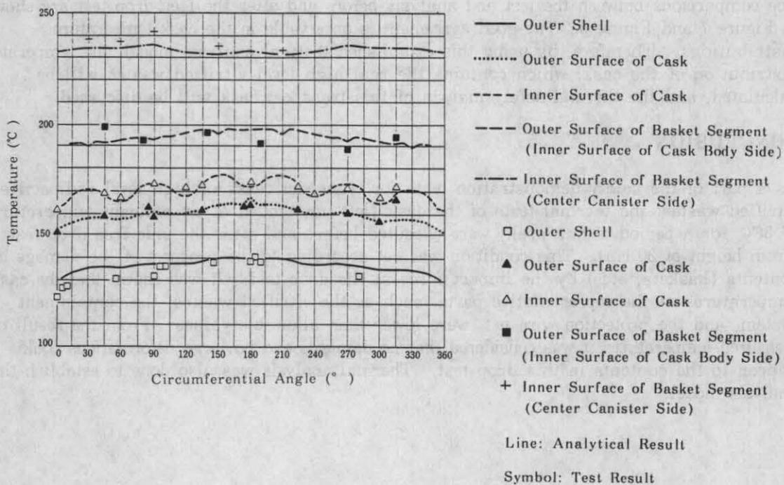
Figure 8. Comparison between Analytical Result and Test Result (after Side Drop Test from 30 cm Height)
