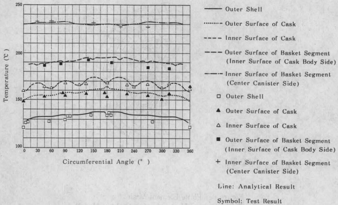
Figure 7. Comparison between Analytical Result and Test Result (before Side Drop Test from 30 cm Height)
