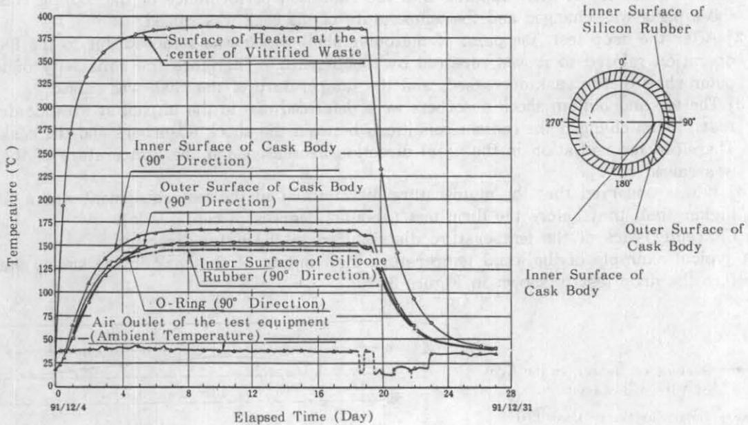
Figure 2. History of Temperature at each part of Transport Cask (After Side Drop Test from 30 cm Height)
