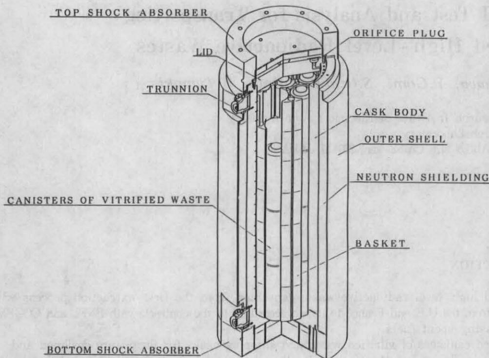
Figure 1. Concept of Transport Cask for Test
