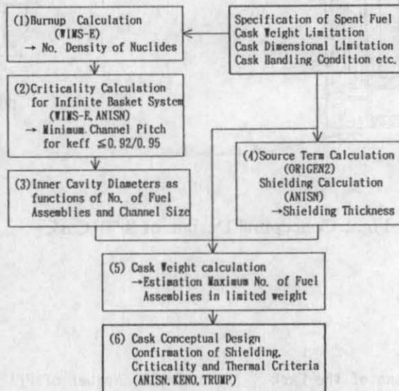
Fig.1 Flow Diagram of the S/T Cask Conceptual Design
