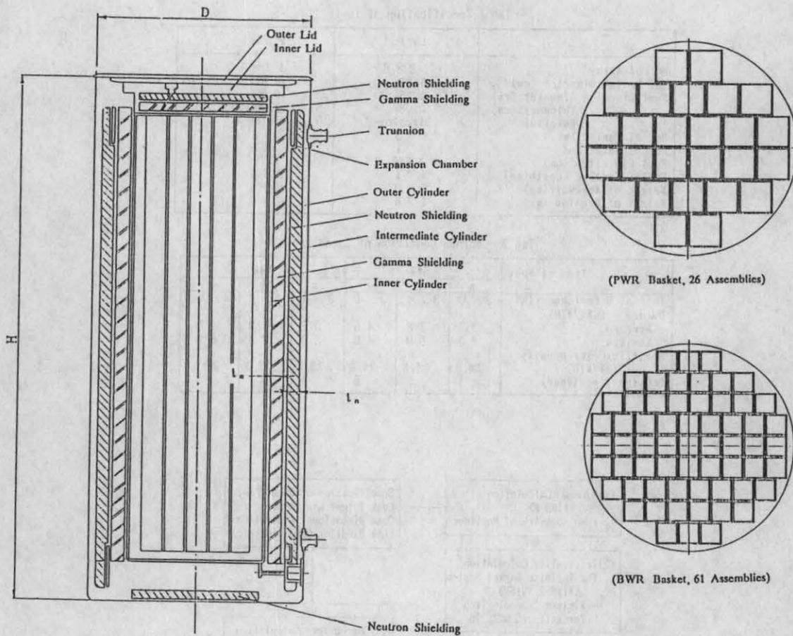
Fig.2 Conceptual Design of S/T Cask
