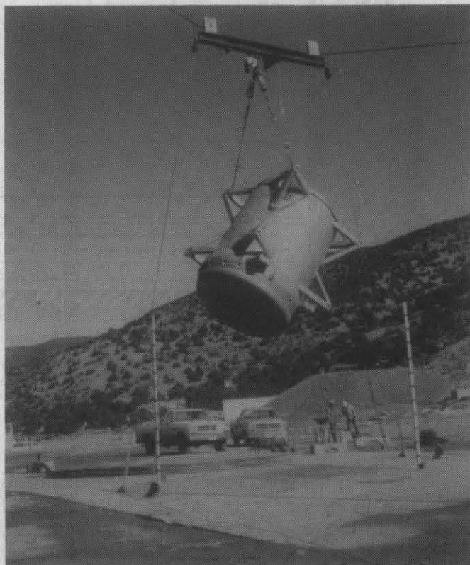
Figure 4. On-Site Container Suspended 3 m Over the Unyielding Target
