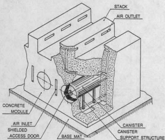
Figure 1 Japanized Horizontal Modular Storage System Arrangement
