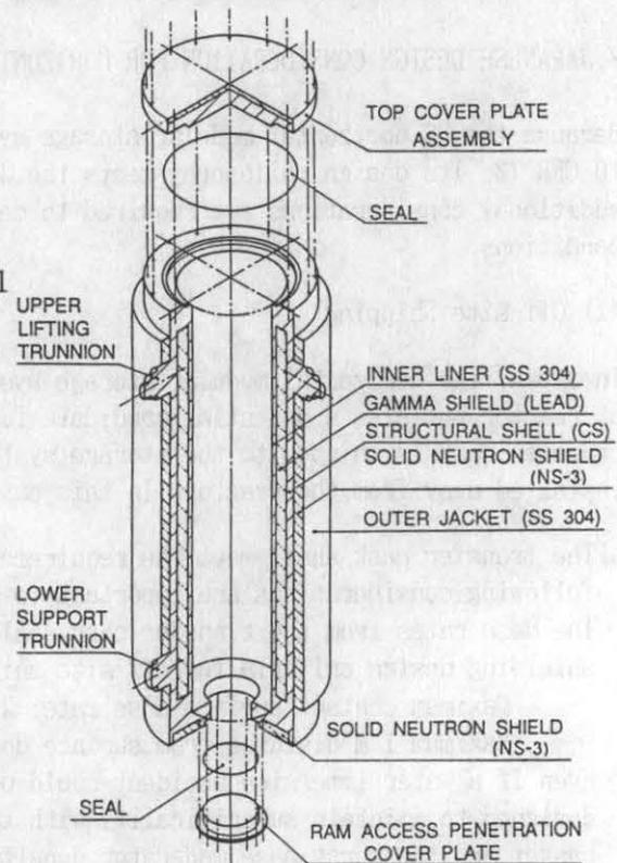
Figure 3 Illustration of Canister Transfer cask
