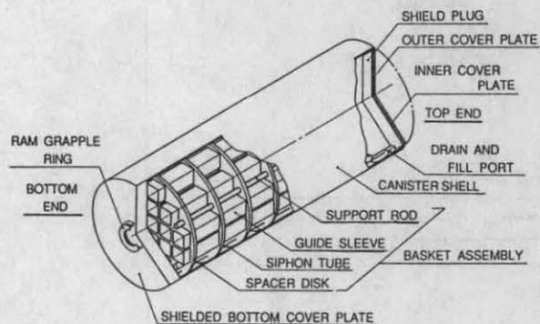
Figure 2 Illustration of PWR Canister
