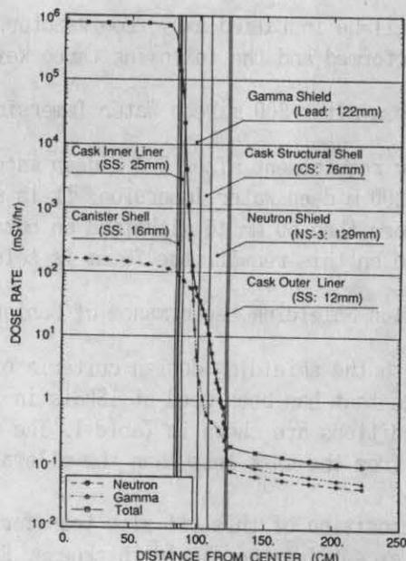
Figure 5 Radiation Dose Rate Distribution Over Cask Radial Direction
