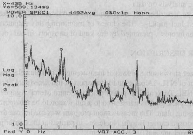
Fig. 1 Power Density Spectrum for vertical acceleration
