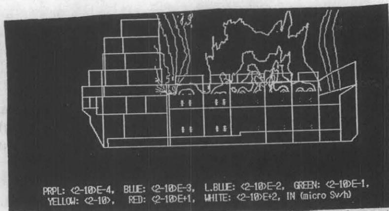
Fig.8 Neutron dose rate distribution in a cask system
