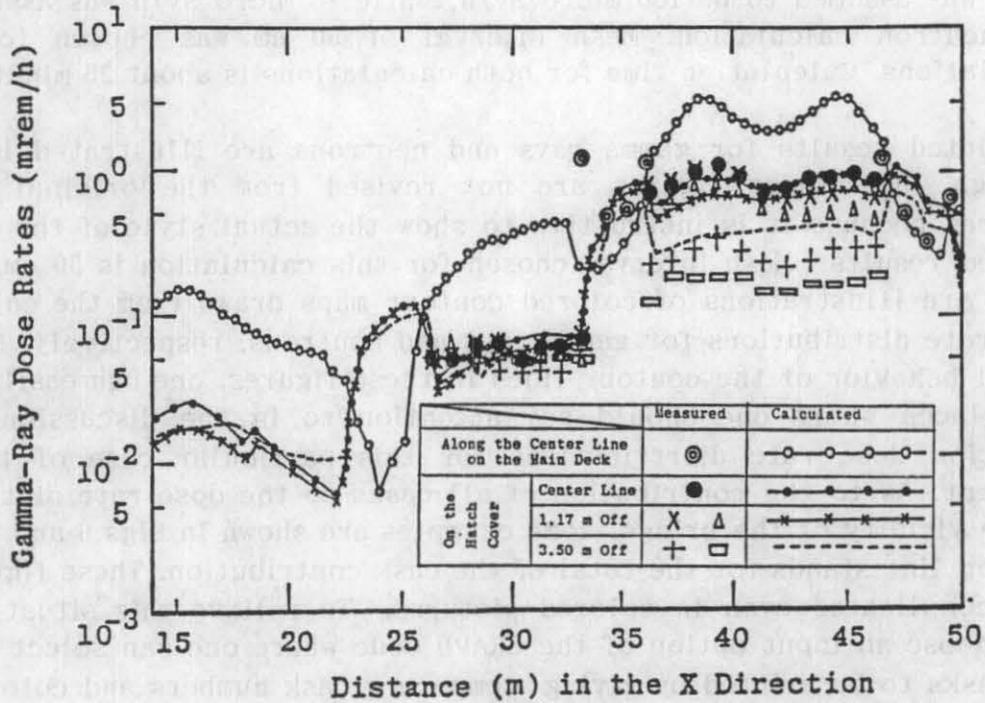
Fig.2 Comparison of dose rate distribution between calculation and measurement
