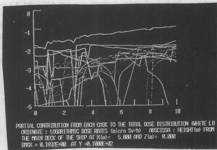
Fig.10 Neutron dose contribution in a cask system
