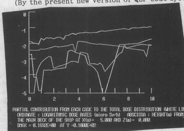
Fig.9 Neutron dose contribution in a cask system
