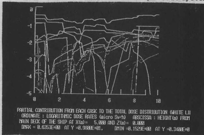
Fig.6 Gamma-ray dose contribution in a cask system
