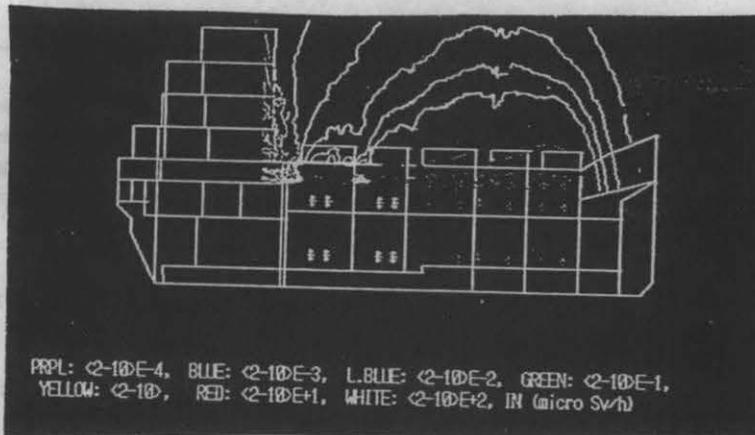
Fig.5 Gamma-ray dose rate distribution in a cask system
