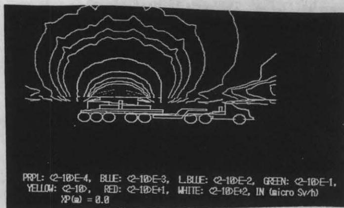
Fig.11 Gamma-ray dose rate distribution in a cask system
