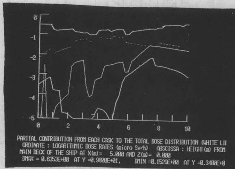
Fig.7 Gamma-ray dose contribution in a cask system
