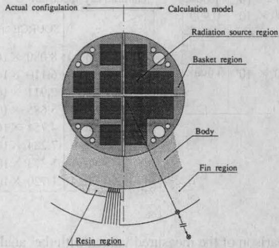
**Fig.5** Dose equivalent rate calculation model
