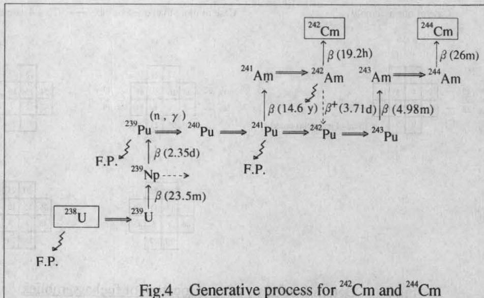
Fig.4 Generative process for <sup>242</sup>Cm and <sup>244</sup>Cm
