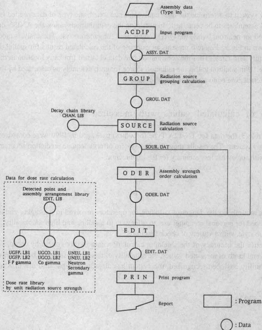
Fig.1 Structural figure of predictive system of cask dose equivalent rate
