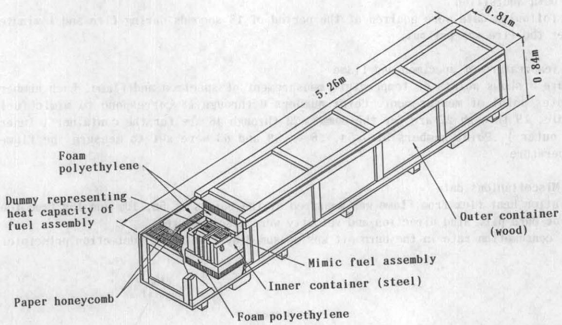
Figure 1 Arrangement of BWR-type specimen
