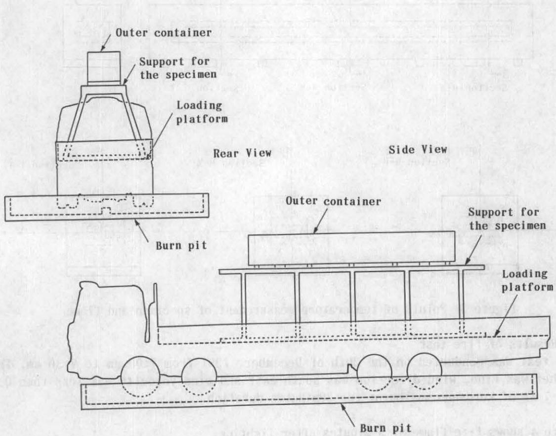
Figure 2 Set up of truck and specimen in the burn pit ( BWR-type )
