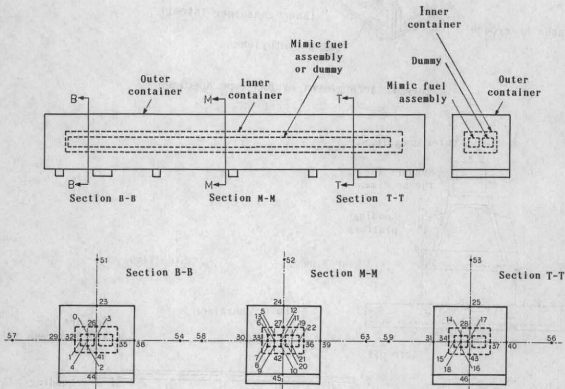
Figure 3 Points of temperature measurement of specimen and flame
