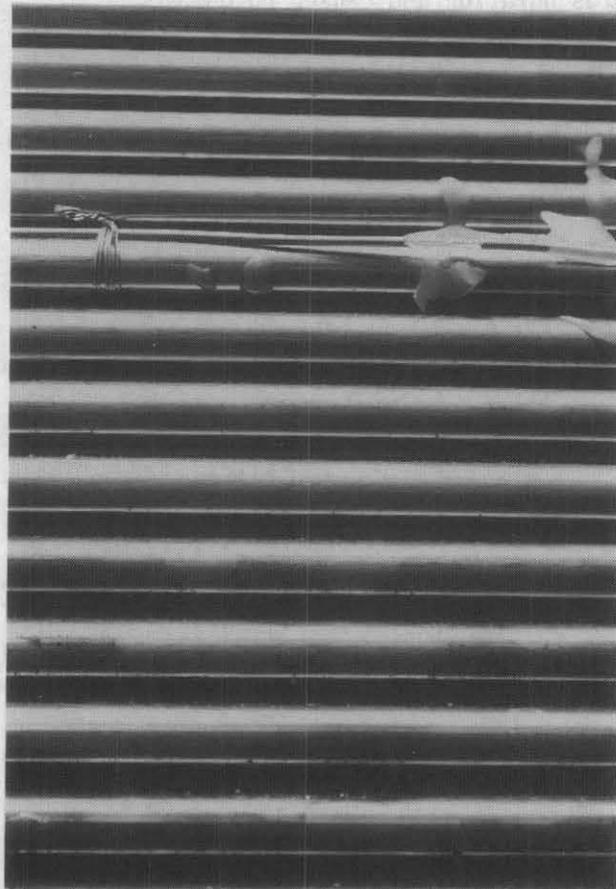
Figure 9 Rods of PWR-type mimic fuel assembly after test
