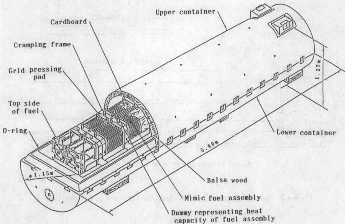
Figure 7 Arrangement of PWR-type specimen
