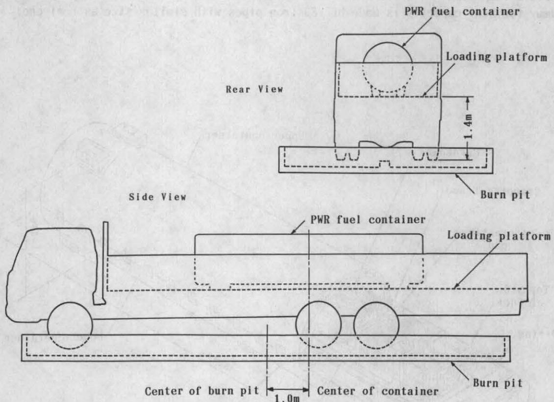
Figure 8 Set up of truck and specimen in the burn pit ( PWR-type )
