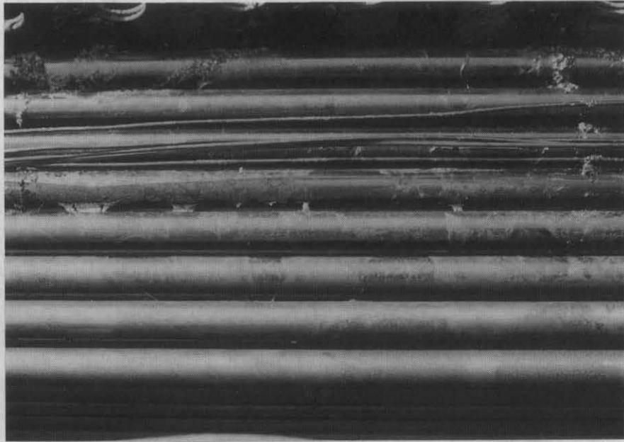
Figure 5 Rods of BWR-type mimic fuel bundle after test
