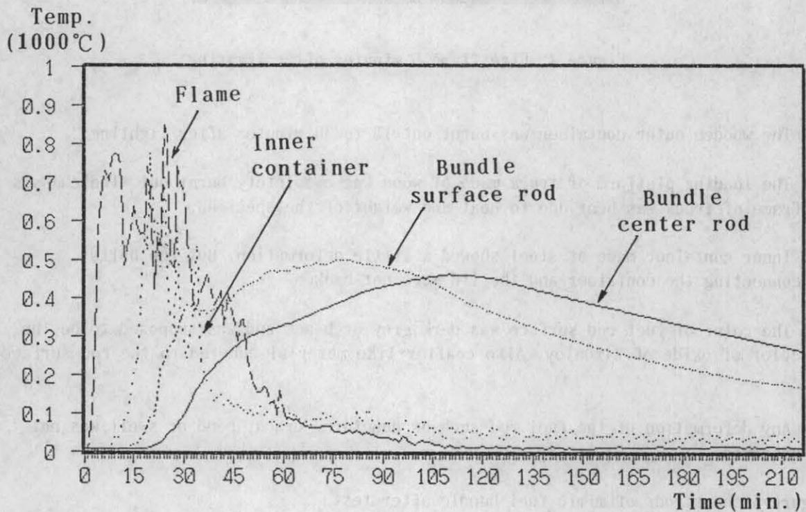
Figure 6 Temperature change of specimen and flame during fire test
