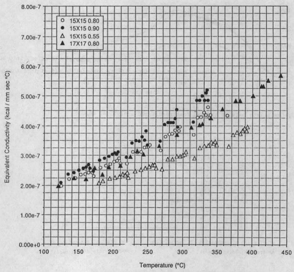
Fig 5. Equivalent conductivity of fuel assembly
