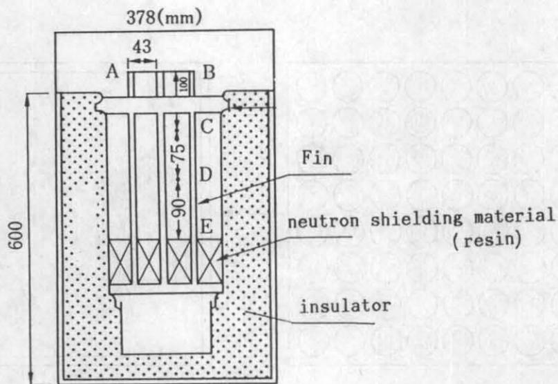
Fig 1. Partial model test body
