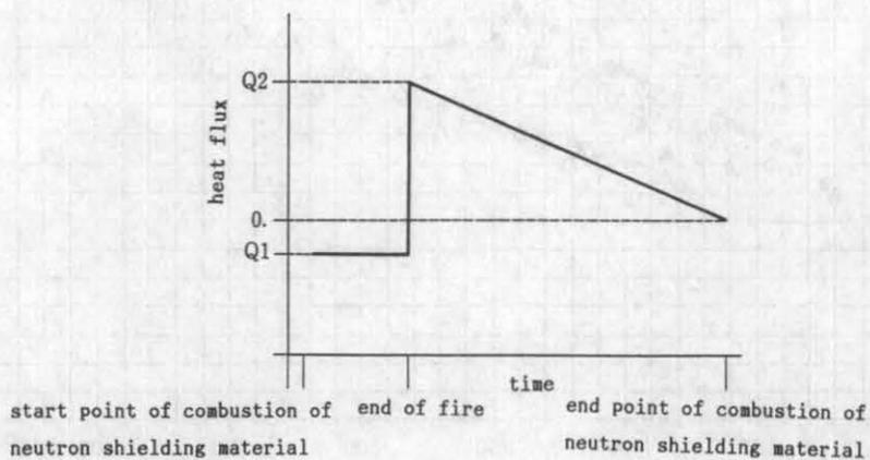
Fig 3. Conceptual drawing of heat flux
