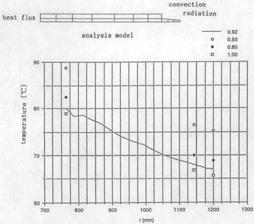
Fig 7. Temperature distribution of simple cask model (finite element method)
