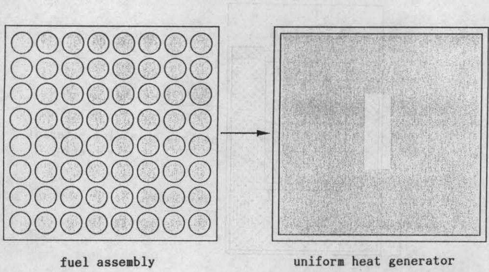
Fig 4. Modeling of the fuel assembly
