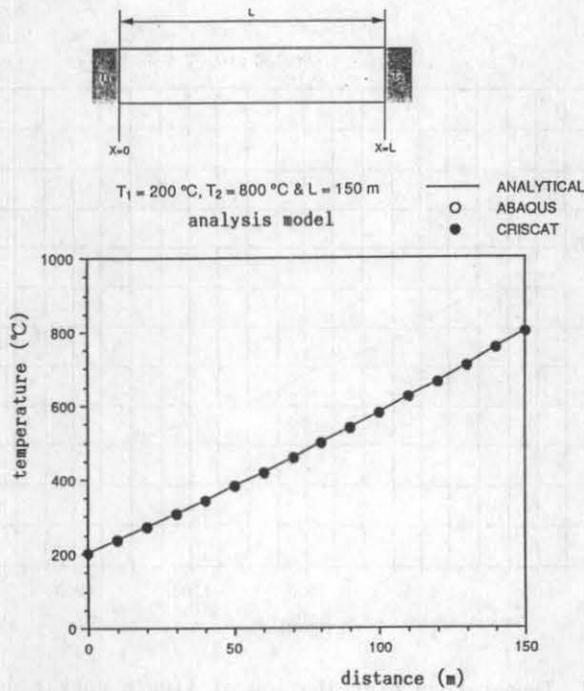
Fig 6. Temperature distribution of one dimensional steel rod
