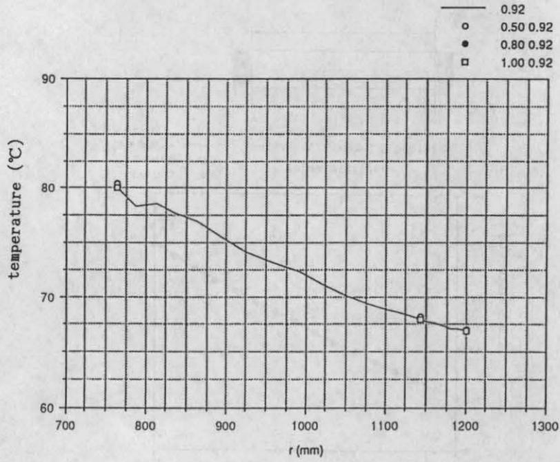
Fig 8. Temperature distribution of simple cask model
