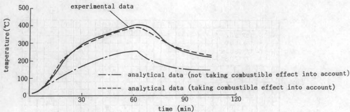
Fig 2. Comparison between thermal test result and analytical result
