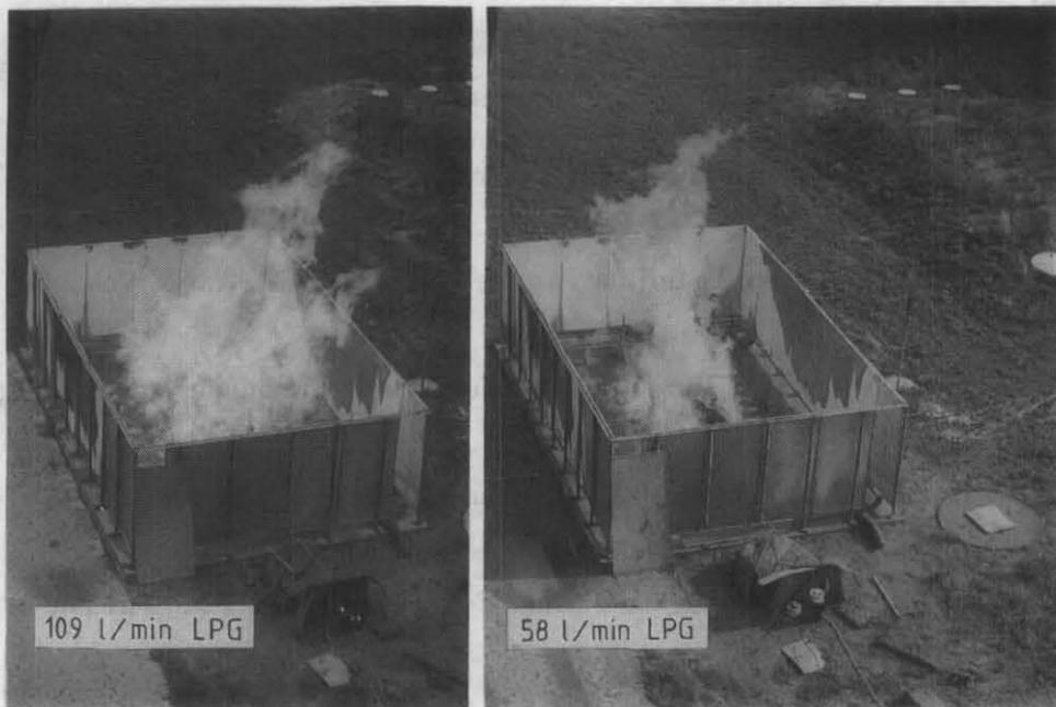
**Figure 9: Flame Characteristic of a High Heat Flux (Left) and a Low Heat Flux (Right) Fire Test**
