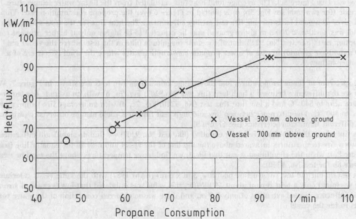
**Figure 6:** Total Average Heat Flux over Propane Consumption Rate
