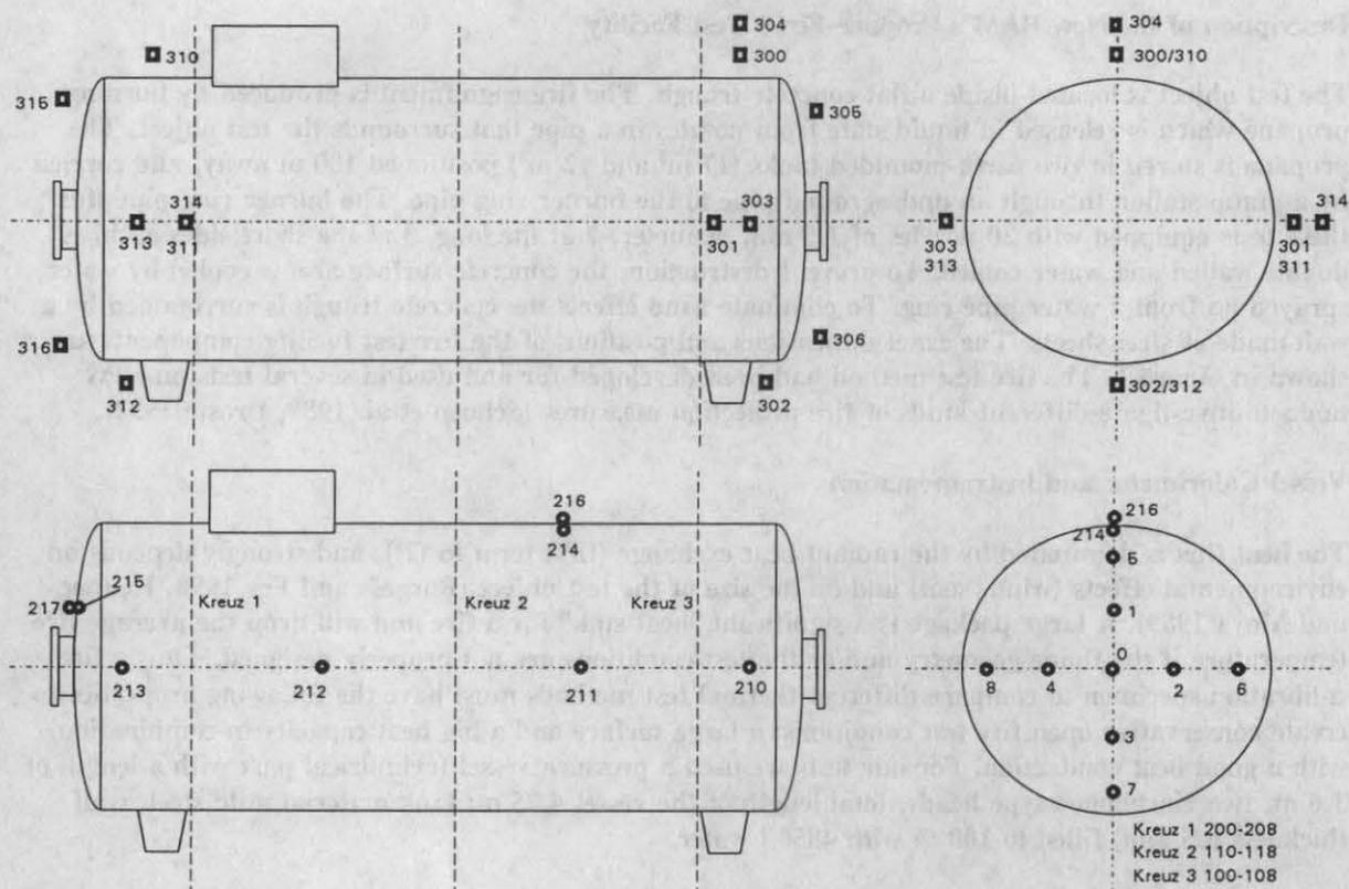
Figure 2: Plan of the Thermocouple Locations
