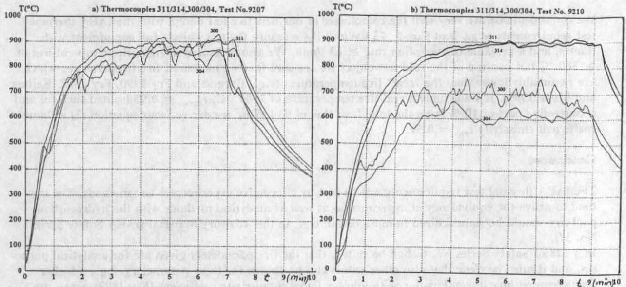
**Figure 8: Fire Temperatures at Equator Line (311, 314) and at Top Line (300, 304) for**
