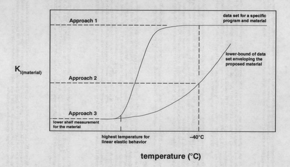
Figure 1. Schematic of the relative values allowed for K<sub>I(material)</sub> for Approaches 1, 2, or 3 for the IAEA revised Appendix IX of Safety Series #37.
