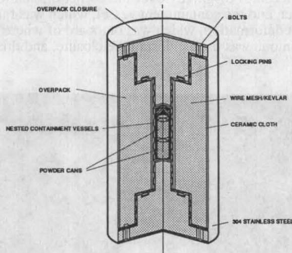
Figure 1. Plutonium Air Transport Package Design Concept
