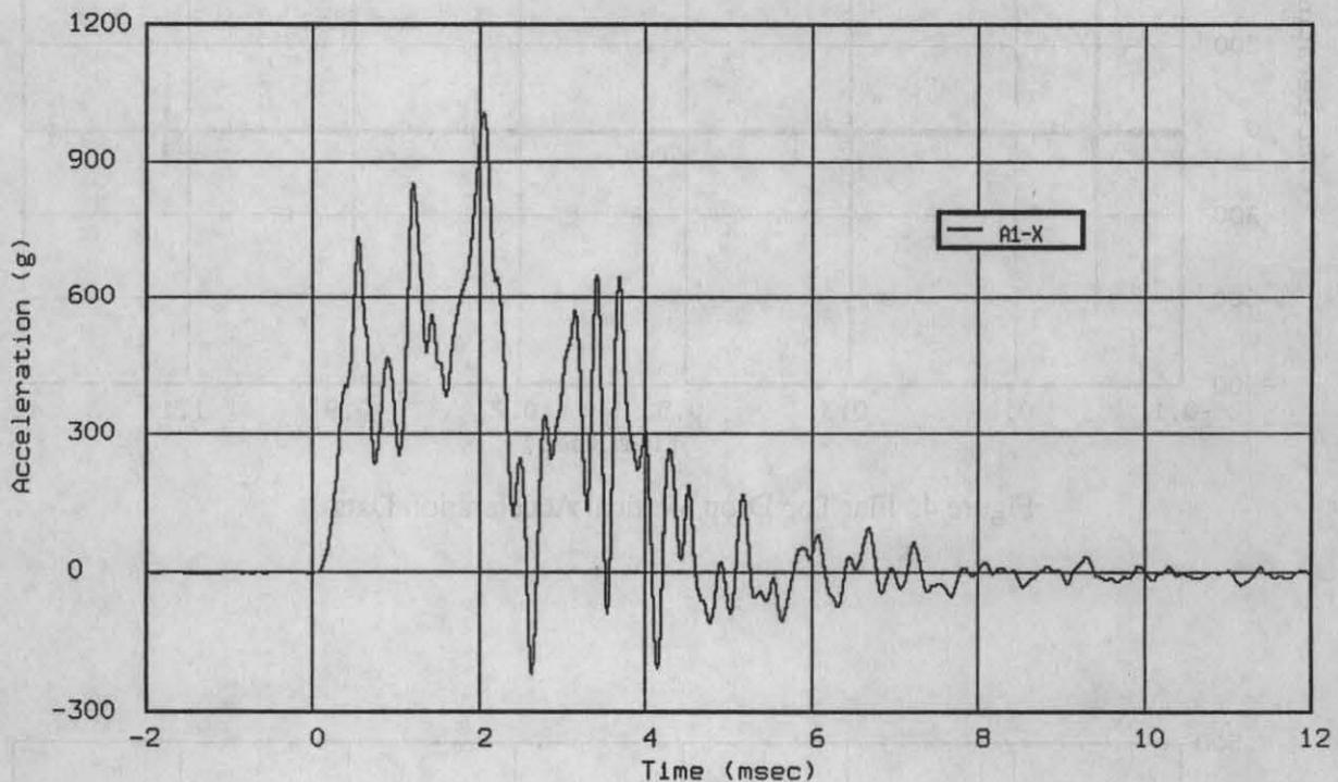
Figure 6. Flat Top Drop Primary Impact Filtered Data
