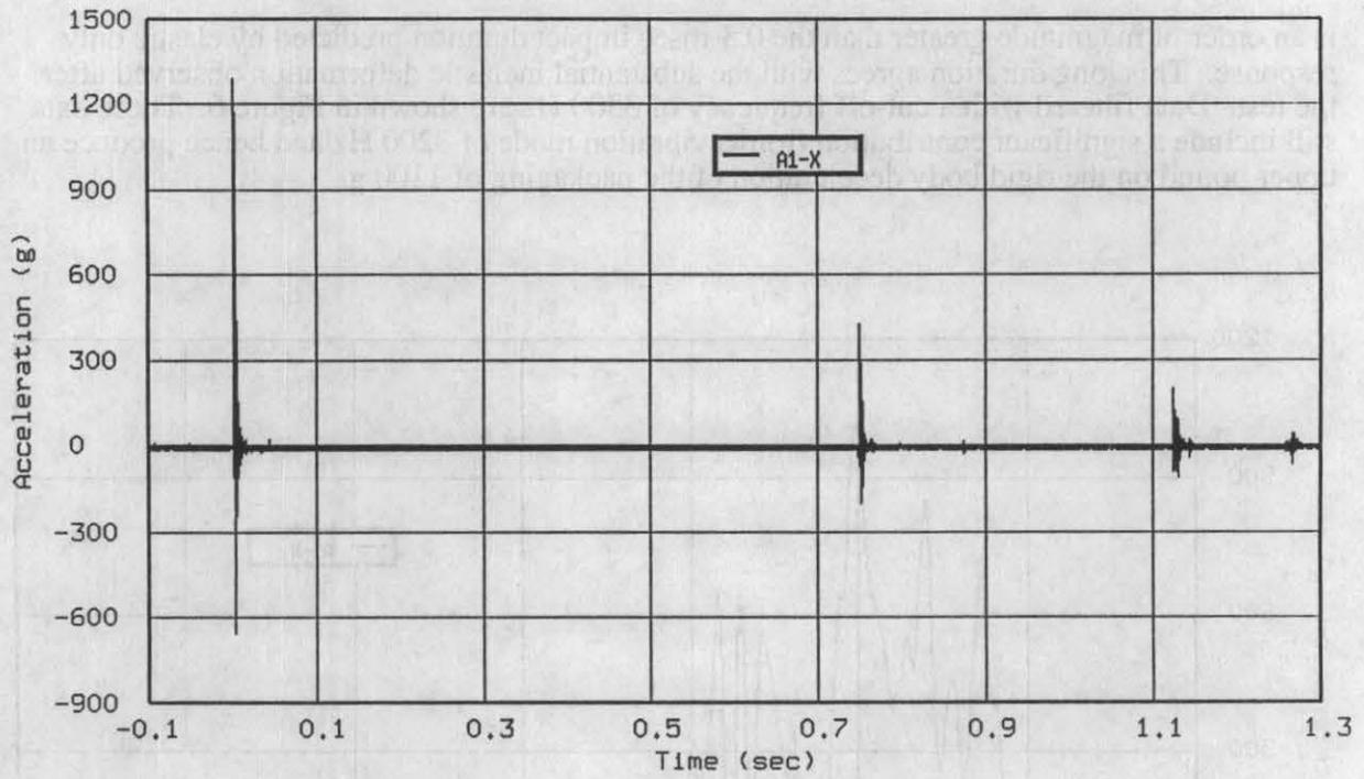
Figure 4. Flat Top Drop Vertical Acceleration Data
