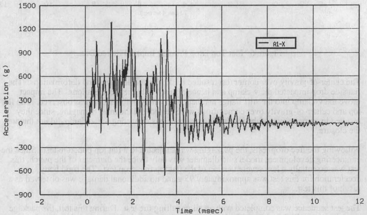
Figure 5. Flat Top Drop Primary Impact Acceleration Data
