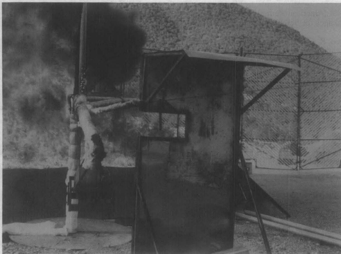
Figure 7. Protective Sample Container Exposed to Ongoing JP-4 Fuel Fire Test
