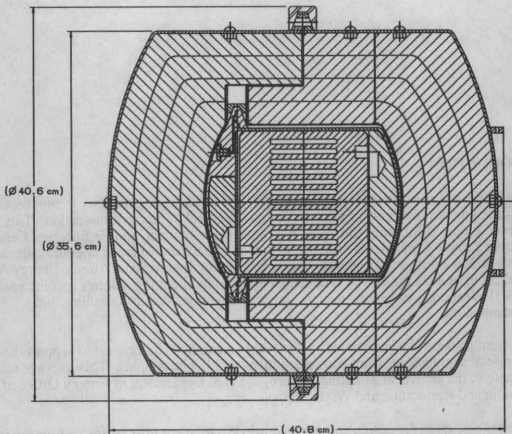
Figure 1. Protective Sample Container Design
