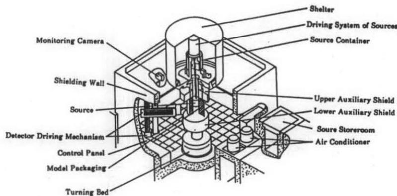
Fig. 3 Bird's-eye View of Shielding Test Facility
