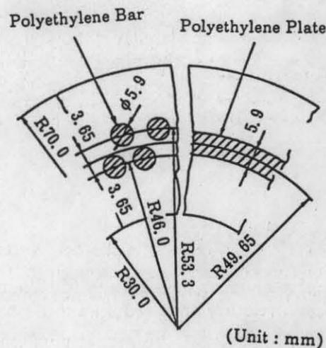
Fig. 2 Relation of Polyethylene Bars and Plates
