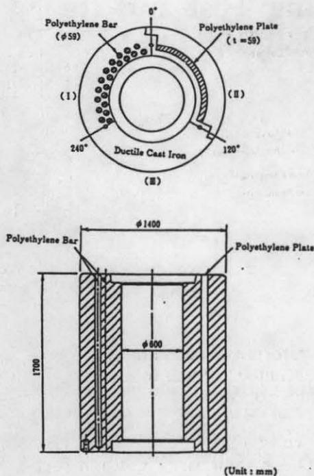
Fig. 1 Configuration of Ductile Cast Packaging Model
