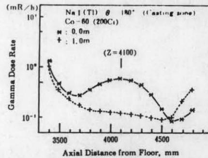
Fig. 6 Axial Gamma Dose Rate Distribution (Na I (Tl), Region (III))
