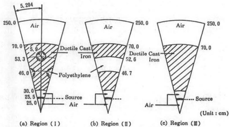
Fig. 8 Model for Shielding Calculation
