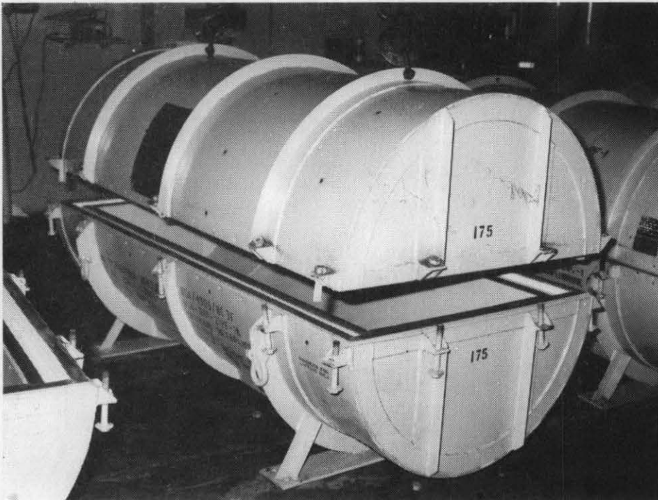
Figure 5. Refurbished USA-DOT 21PF-1A Overpack.
