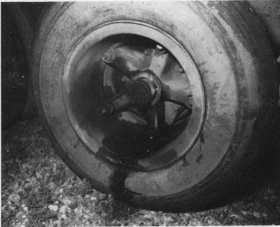
Figure 4. Leaking Wheel Seal of Equipment Rejected from Loading.
