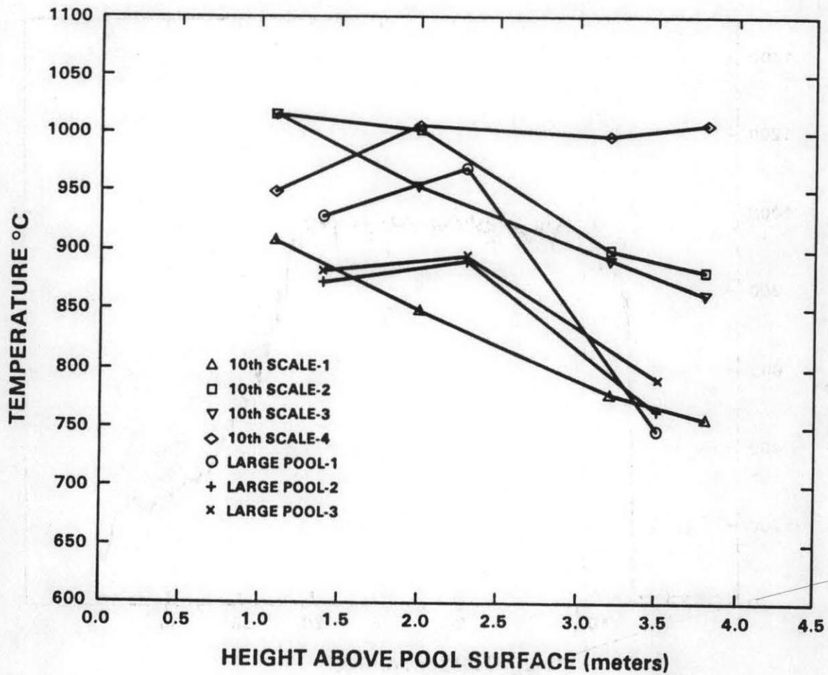
**Average Temperatures in the 10th Scale Facility and the 9 meter x 18 meter Open Pool Facility**
