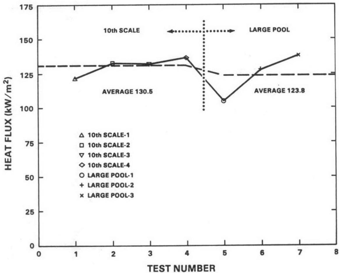
**Average Cold Wall Heat Fluxes in the 10th Scale Facility and the 9 meter x 18 meter Open Pool Facility**
