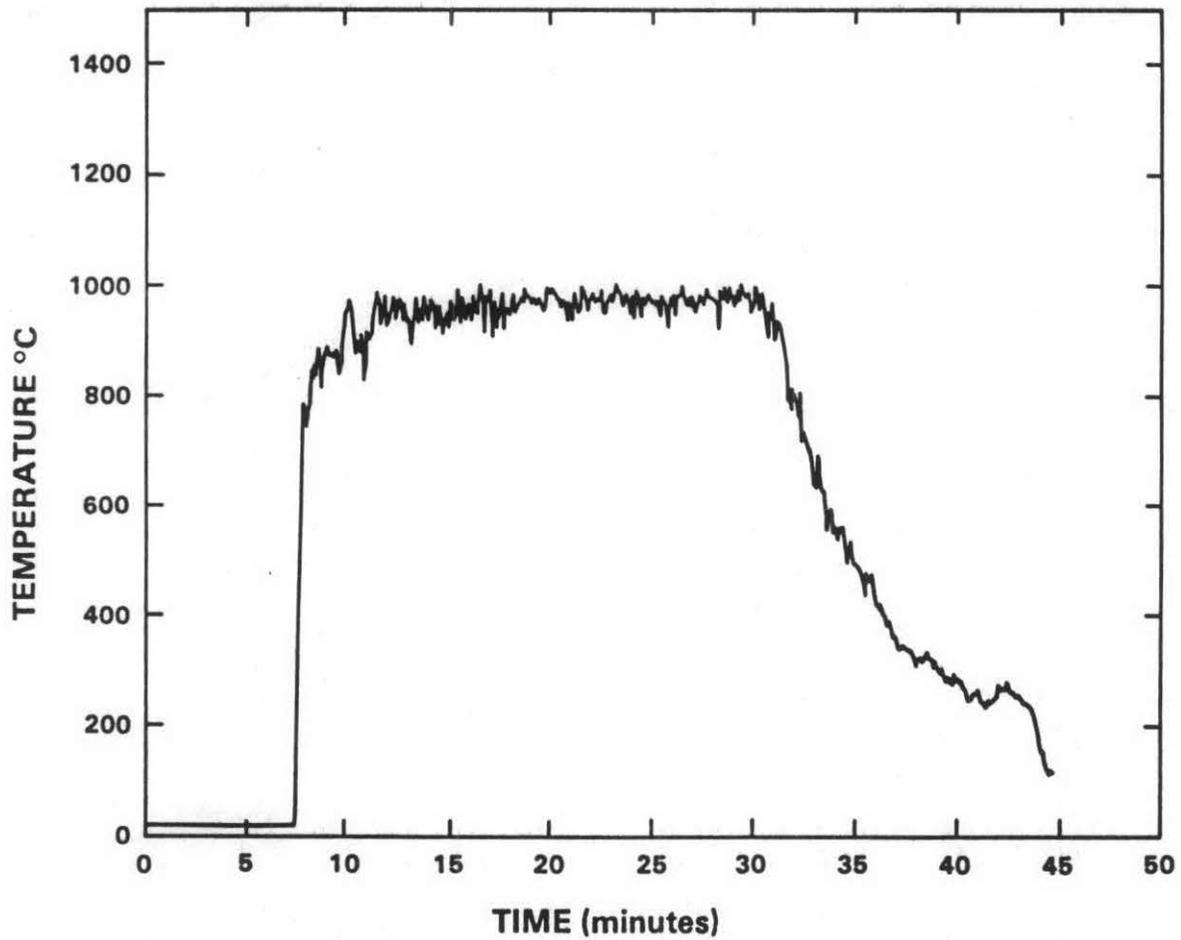
**Temperature History at 3.2 meters During a Test in the 10th Scale (Wind Shielded Facility) Average: 954°C, Standard Deviation: 17°C**
