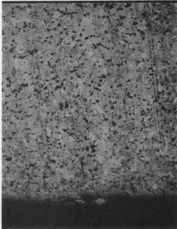
Figure 3 Photomicrograph of creep specimen at the fracture zone.
