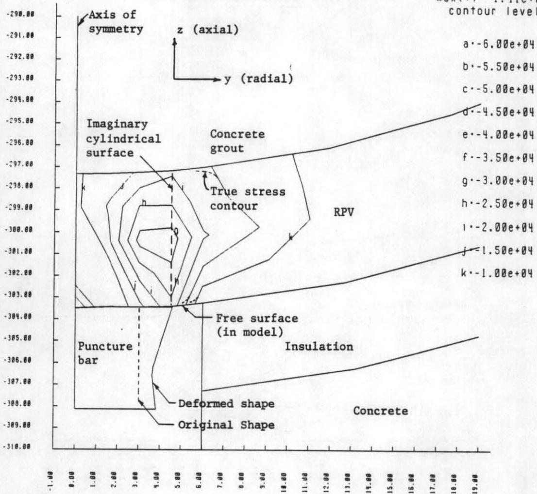
Fig. 2. Contours of y-z shear stress at time of 19 ms.
