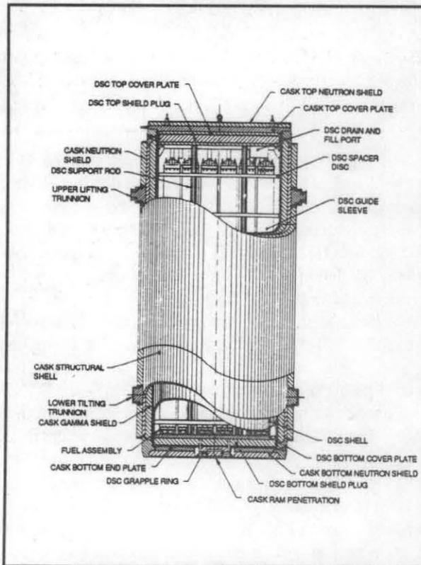
Figure 2 Composite View of NUHOMS®-24P Cask, Canister, and Fuel
