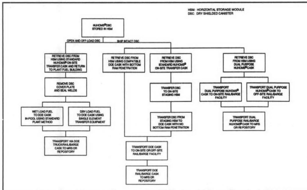
Figure 4 Options for Away-From-Reactor Shipment of Spent Fuel with NUHOMS® System
