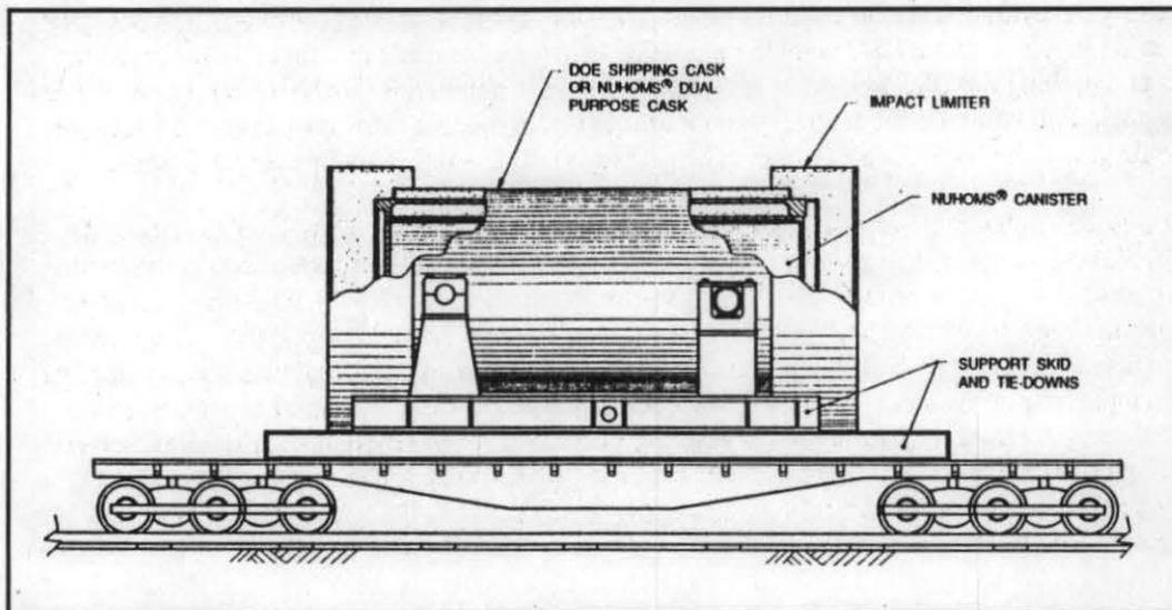
Figure 7 OCRWM Cask or Dual Purpose NUHOMS® Cask and Canister Secured for Shipment on Rail Car
