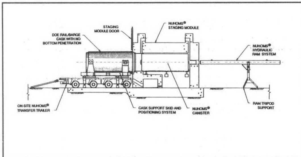
Figure 8 NUHOMS® Canister Transfer From Staging Module to OCRWM Cask
