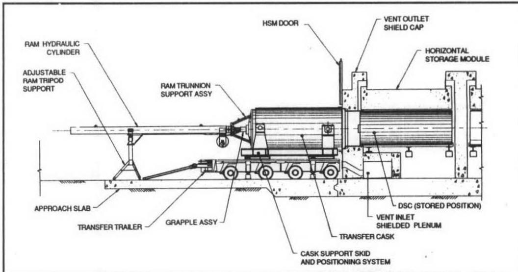
Figure 3 Standard NUHOMS®-24P System Components, Structures, and Transfer Equipment
