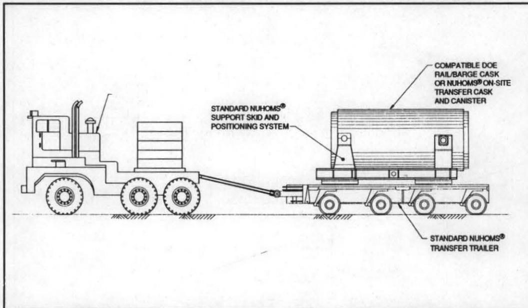
Figure 5 On-Site Transport of Cask/NUHOMS® Canister to Staging Module or Rail/Barge Facility
