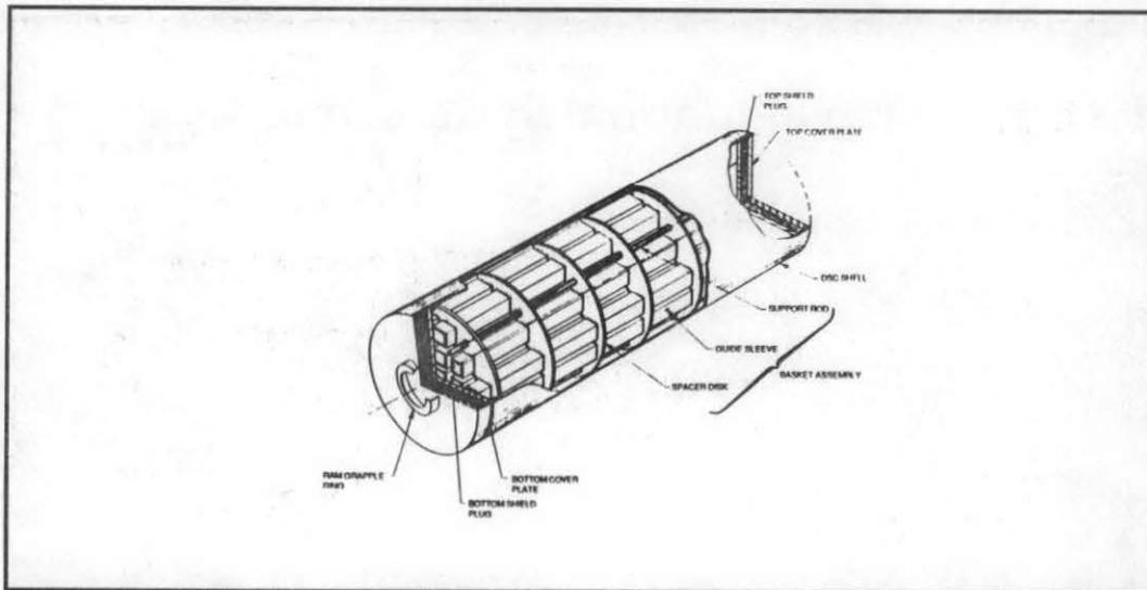
Figure 1 NUHOMS®-24P Dry Shielded Canister
