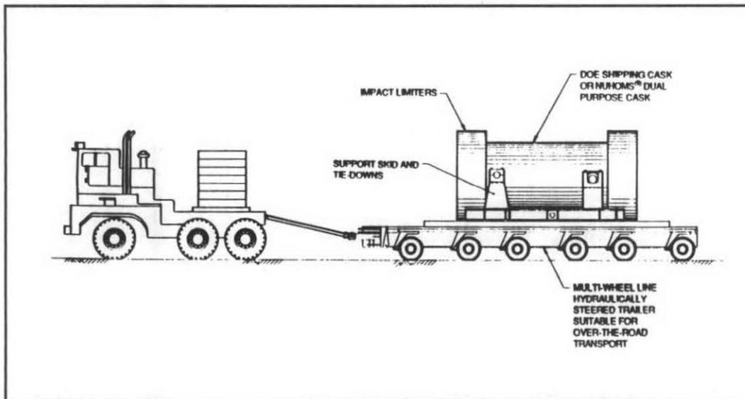
Figure 6 Off-Site Transport of OCRWM or Dual Purpose NUHOMS® Canister to Rail/Barge Facility
