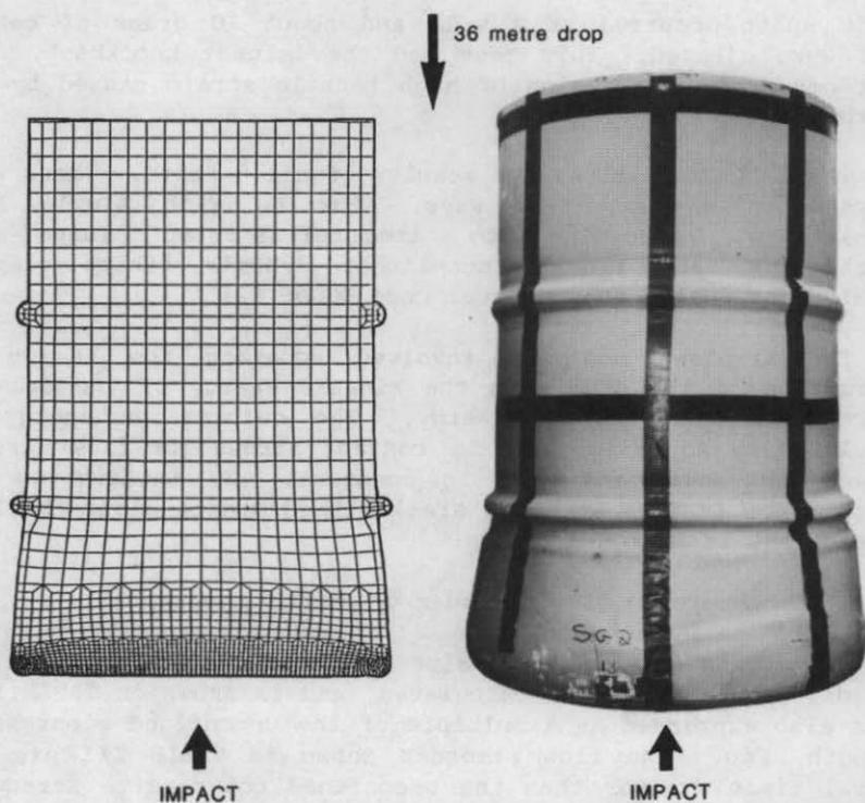
FIG. 4. Comparison of actual and calculated deformations for axis vertical drum drop.
