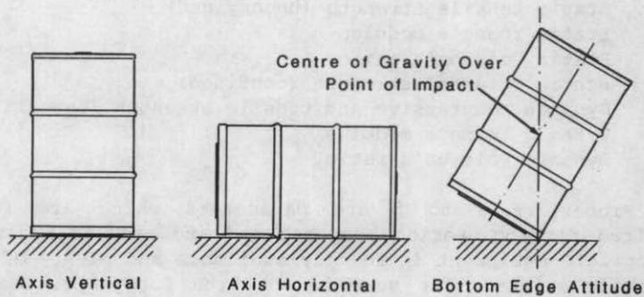
FIG. 1. Drum drop test attitudes.
