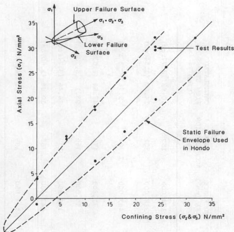
FIG. 3. Magnox sludge triaxial test results and HONDO failure envelope.
