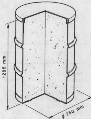
FIG. 2. The 500 L test drum.
