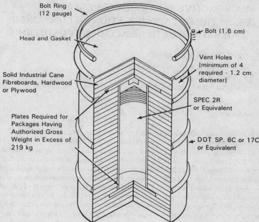
FIG. 1. DOT Specification 6M container.
