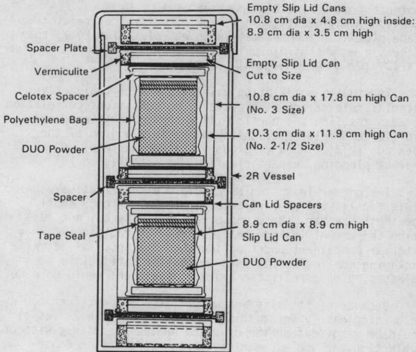
FIG. 2. Packaging configuration for DUO powder inside a 6M container.
