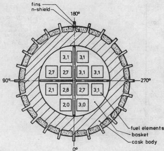
FIG. 2 TN 1300 hot demonstration — Thermal power distribution in the basket.
