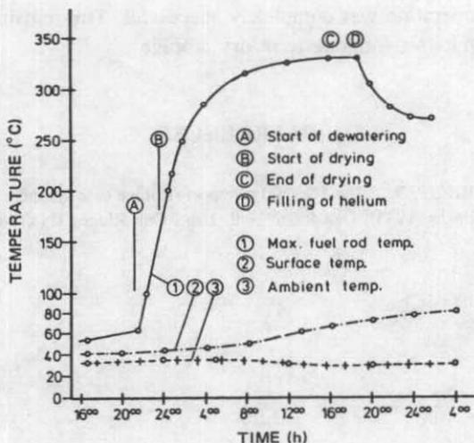
FIG. 3 TN 1300 hot demonstration — main temperatures.
