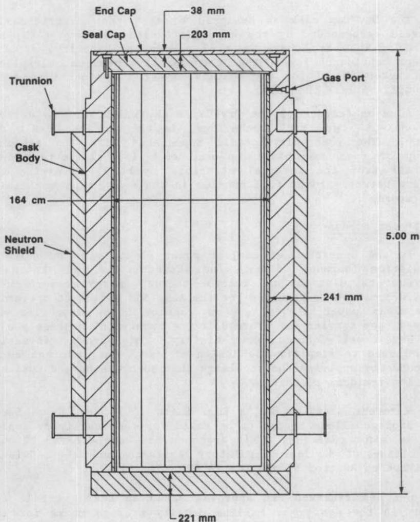
FIG. 1. The Dry-Cap spent fuel storage cask.
