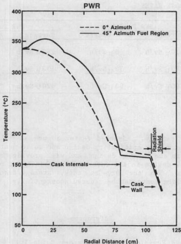
FIG. 3. Radial cask temperature profiles.
